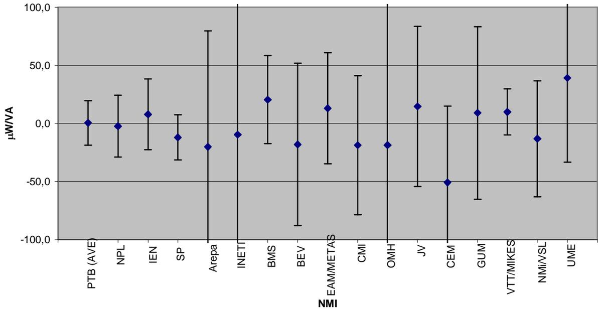
**Figure 8. Deviation from Reference Value 120 V, 5 A, PF 0.5 Lag ( $k=2$ )**
