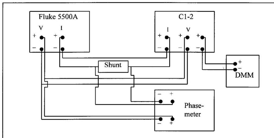
Fig 5.1 Schematic diagram of the Arepa measuring system.
