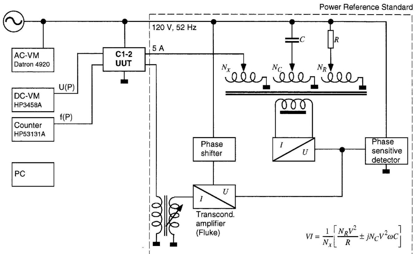
Fig 9.1 Schematic diagram of the METAS measuring system.
