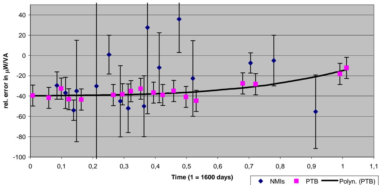
Figure 4. Reported results, 120 V, 5 A, PF = 0.0 Lead (cap) ( $k = 1$ )
