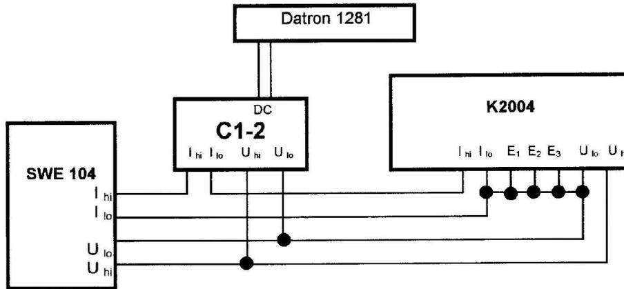
Fig 8.1 Schematic diagram of the BEV measuring system.
