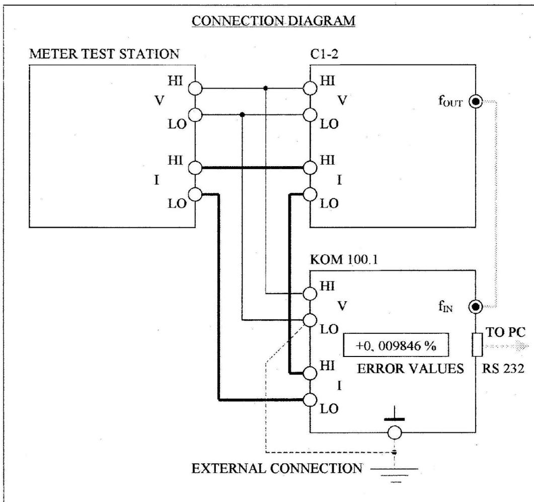
Fig 14.1 Schematic diagram of the GUM measuring system.
