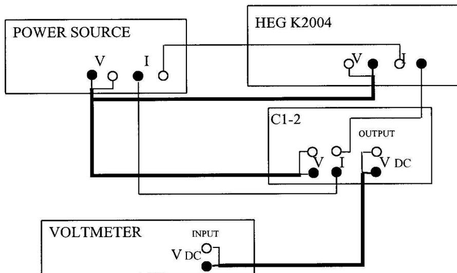
Fig 13.1 Schematic diagram of the CEM measuring system.
