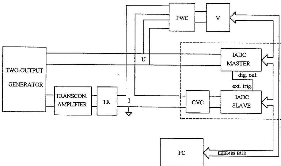
Fig 3.1 Schematic diagram of the IEN measuring system.
