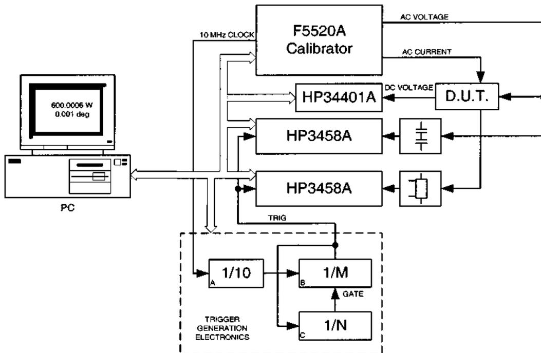
Figure 15.1: Measurement principle. DMMs are triggered simultaneously.  $N$  is the number of samples and  $M$  determines the triggering frequency.
