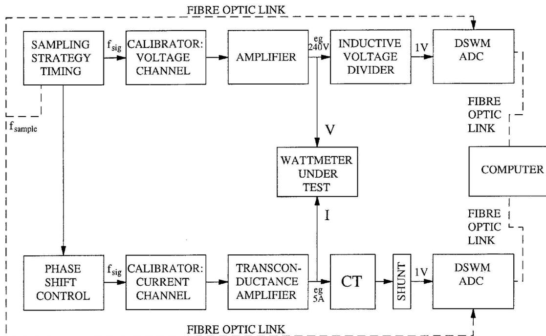
Fig 2.1 Schematic diagram of the NPL measuring system.
