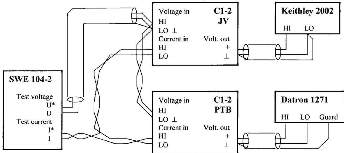
Fig 12.1 Schematic diagram of the JV measuring system.
