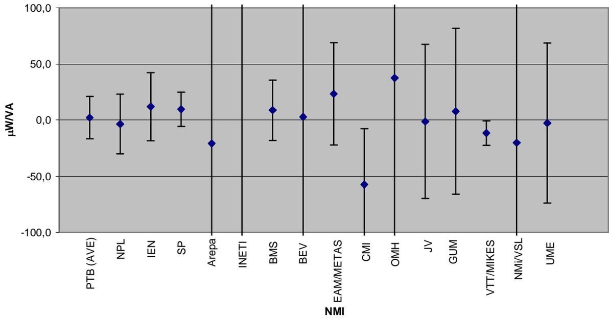
Figure 10. Deviation from Reference Value 120 V, 5 A, PF 0.0 Lag ( $k=2$ )
