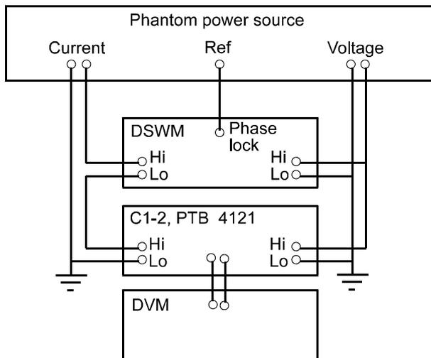
Fig 4.1 Schematic diagram of the SP measuring system.
