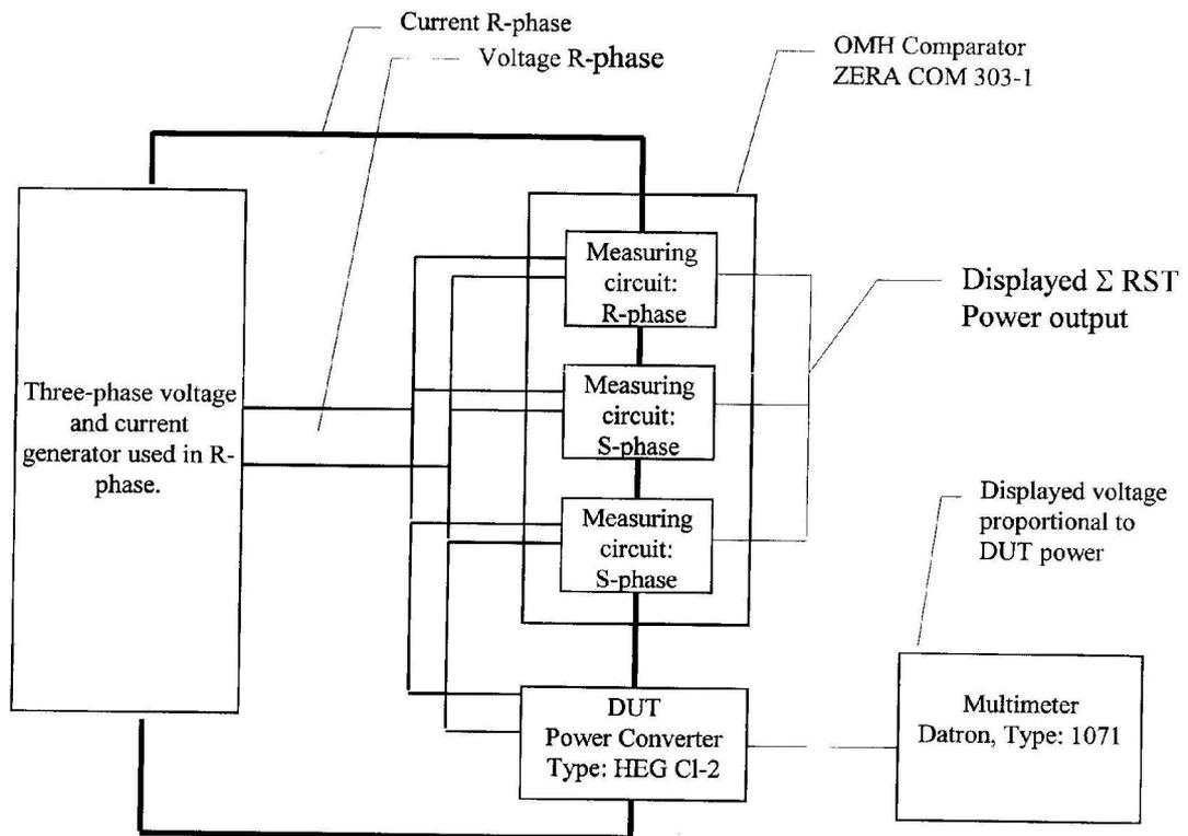
Fig 11.1 Schematic diagram of the OMH measuring system.
