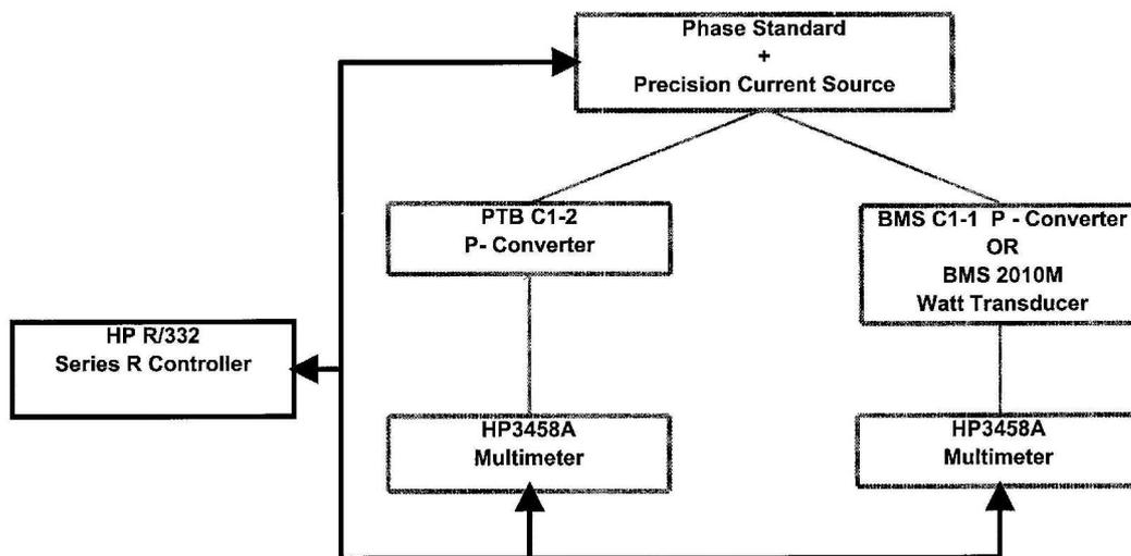
Fig 7.1 Schematic diagram of the BMS measuring system.
