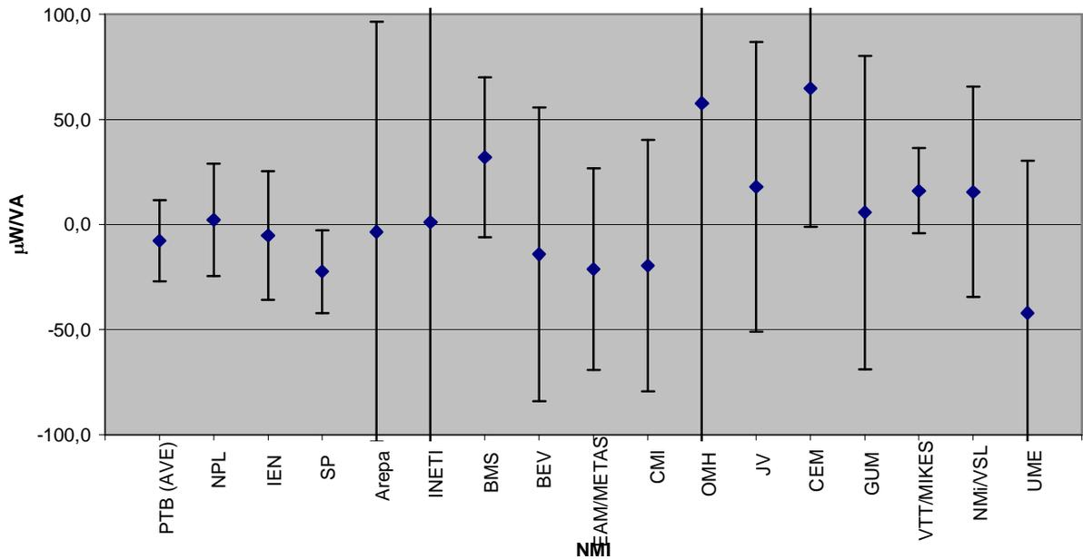
Figure 9. Deviation from Reference Value 120 V, 5 A, PF 0.0 Lead ( $k=2$ )
