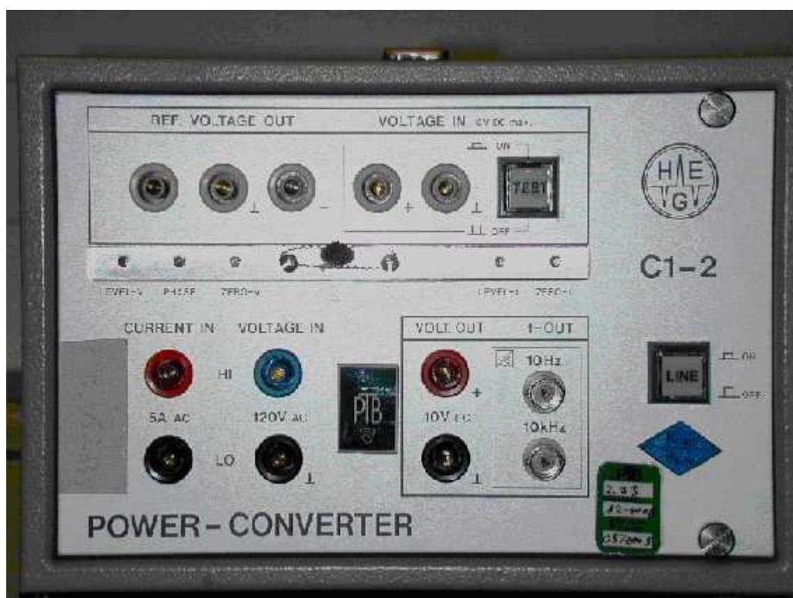
**Figure 1.** Front panel of the travelling standard C1-2.
