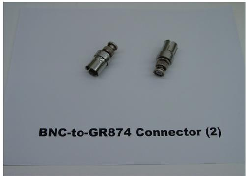
Figure I8. BNC-to-GR874 connectors
