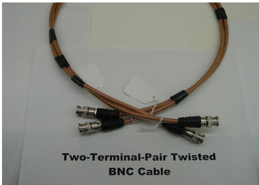
Figure I11. Two-terminal-pair twisted BNC cable
