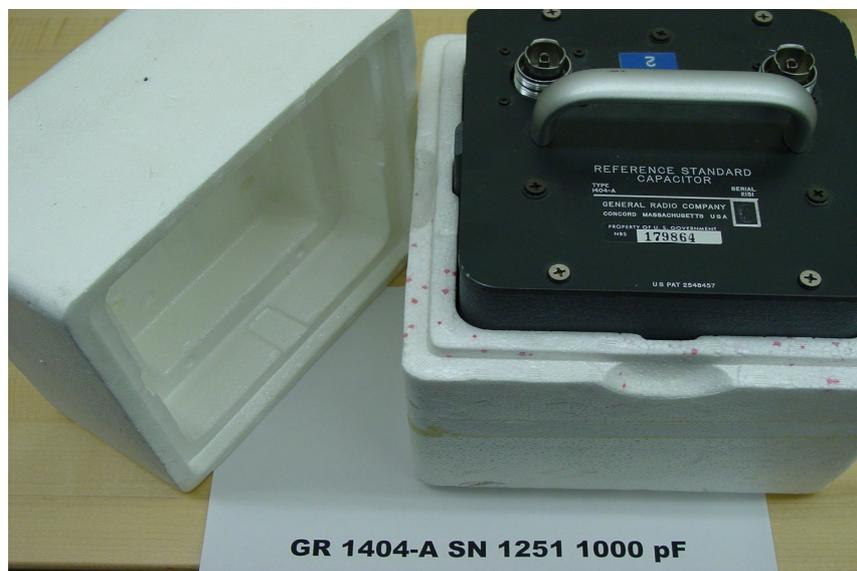
Figure I4. GR1404-A Capacitance Standard in foam carton
