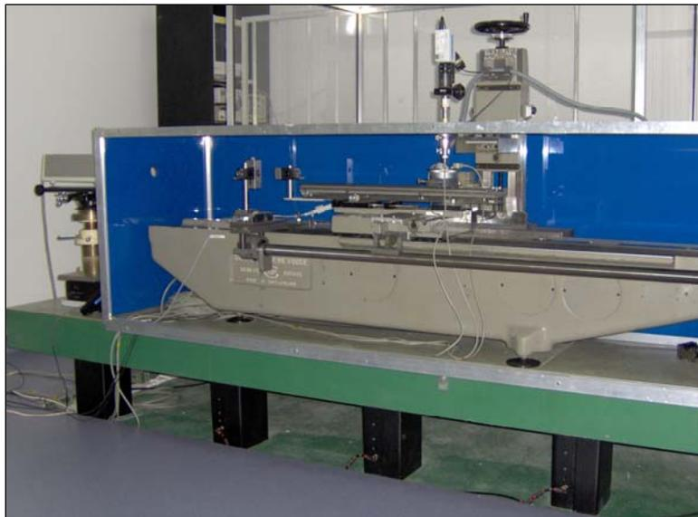
The environmental parameters (material and air temperature) were measured by interferometer sensors. Humidity was measured with thermo-hygrometer LB-706. The refractive index of air was calculated from the modified Edlen formula [G. Bönsch and E. Potulski, *Metrologia*, 1998, 35] with sensors corrections.
