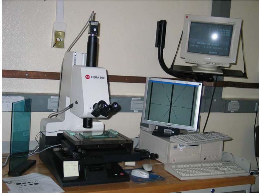
The measurement range of the instrument is 150 mm x 100 mm, and the minimal division of the microscope scale is 0,1  $\mu\text{m}$
