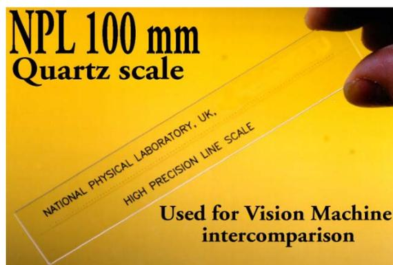
Fig. 2: NPL line scale
