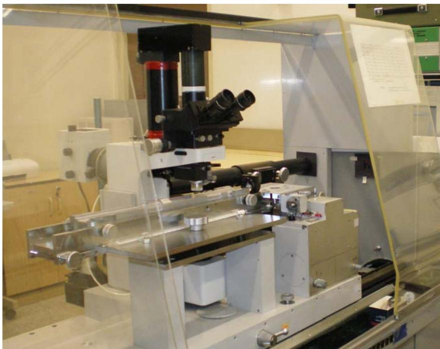
Figure 1: The laser line width measurement system
