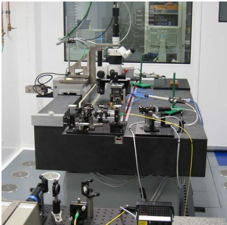
Figure 1. MIKES' line scale interferometer
