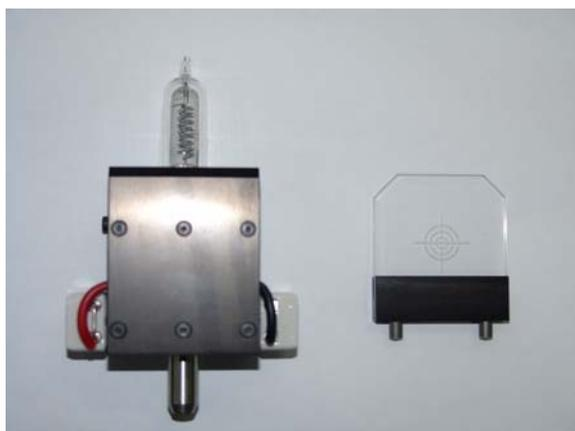
Figure 3-1. Transfer standard lamp and alignment jig.
