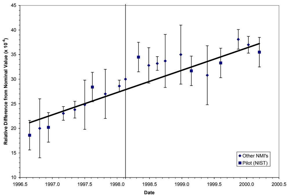
**Figure 3.** Measurements of 10 MΩ standard S/N HR7552 by all participants. Error bars denote individual NMI's expanded relative uncertainty using  $k = 2$ . Least-squares linear regression line based only on the pilot laboratory measurements.
