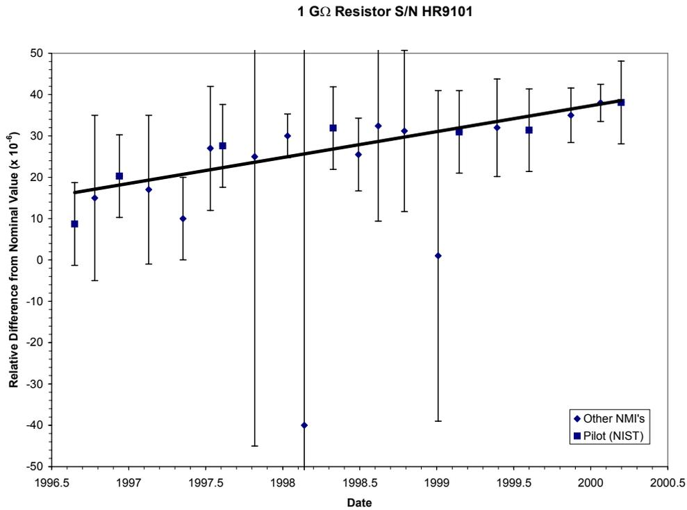
**Figure 5.** Measurements of 1 G $\Omega$  standard S/N HR9101 by all participants. Error bars denote individual NMI's expanded relative uncertainty using  $k = 2$ . Least-squares linear regression line based only on the pilot laboratory measurements.
