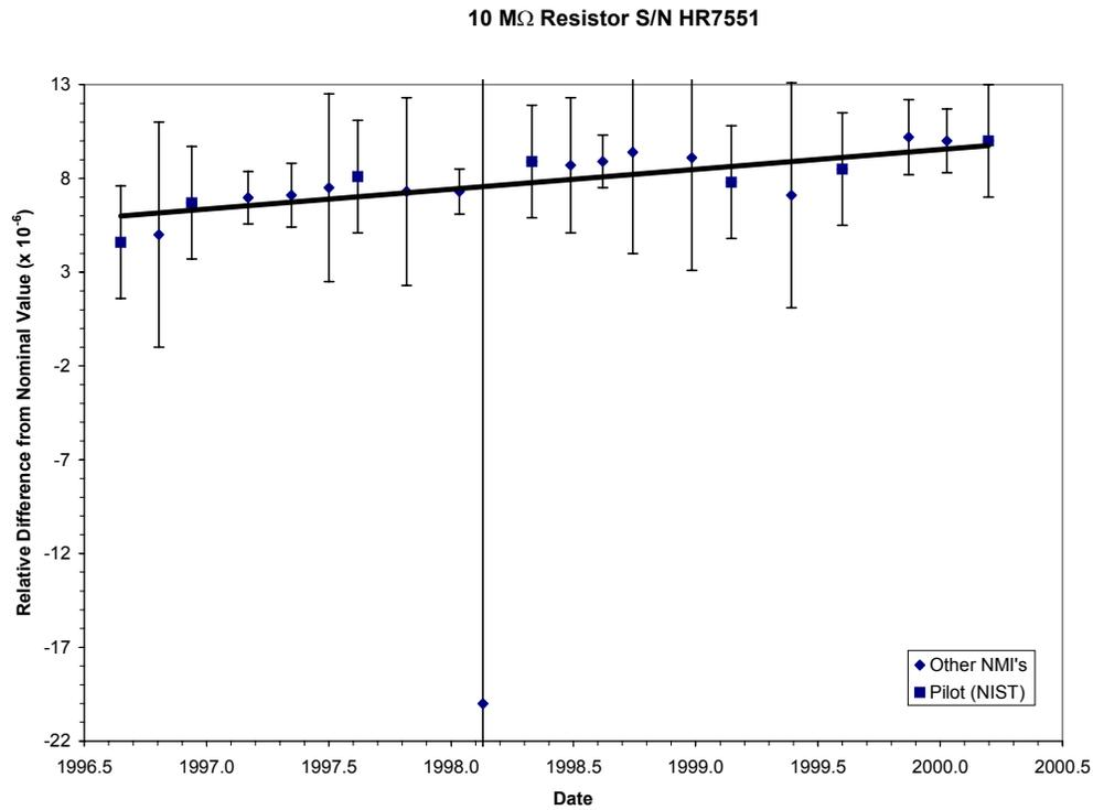
**Figure 2.** Measurements of 10 M $\Omega$  standard S/N HR7551 by all participants. Error bars denote individual NMI's expanded relative uncertainty using  $k = 2$ . Least-squares linear regression line based only on the pilot laboratory measurements.
