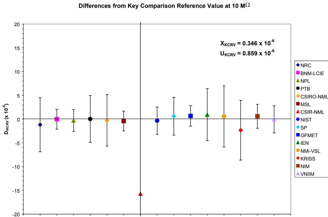
**Figure 4.** Differences from key comparison reference value,  $D_{iKCRV}$ , at 10 M $\Omega$ . Error bars denote  $\pm$  expanded relative uncertainty,  $U_{iKCRV}$ , for the individual NMIs using  $k = 2$ , which includes the  $U_{KCRV}$ .
