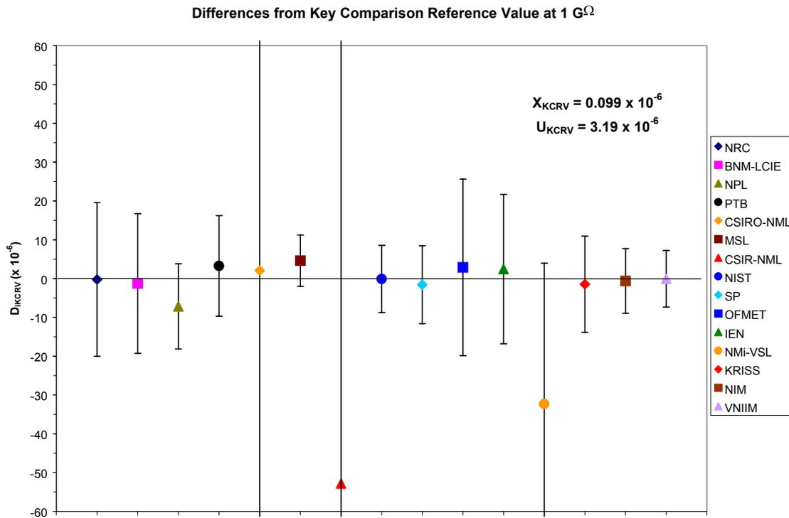
**Figure 8.** Differences from key comparison reference value,  $D_{iKCRV}$ , at 1 GΩ. Error bars denote  $\pm$  expanded relative uncertainty,  $U_{iKCRV}$ , for the individual NMIs using  $k = 2$ , which includes the  $U_{KCRV}$ .
