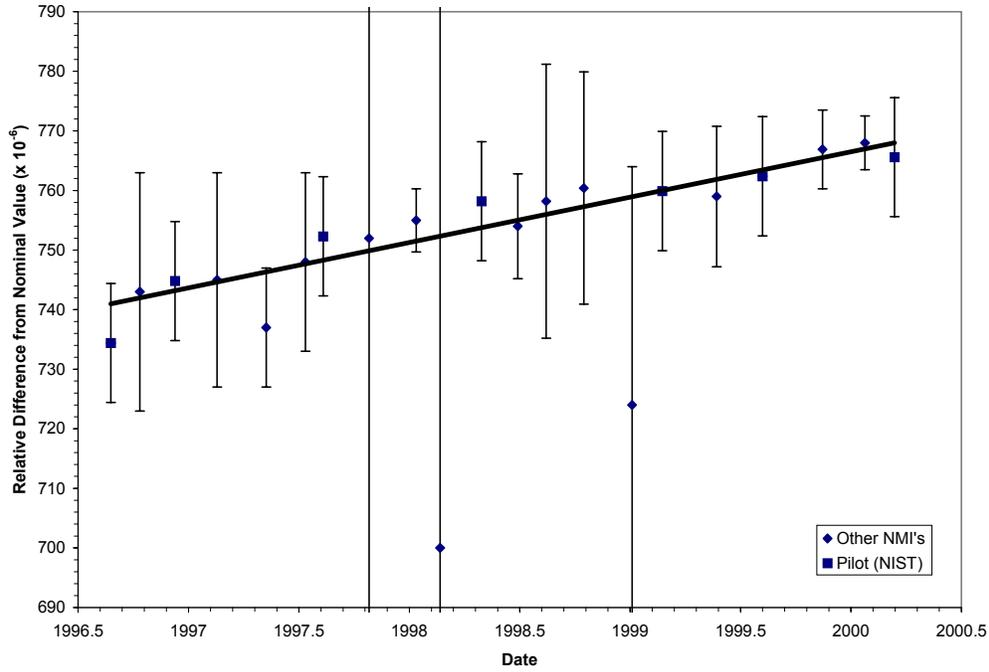
**Figure 7.** Measurements of 1 GΩ standard S/N HR9106 by all participants. Error bars denote individual NMI's expanded relative uncertainty using  $k = 2$ . Least-squares linear regression line based only on the pilot laboratory measurements.
