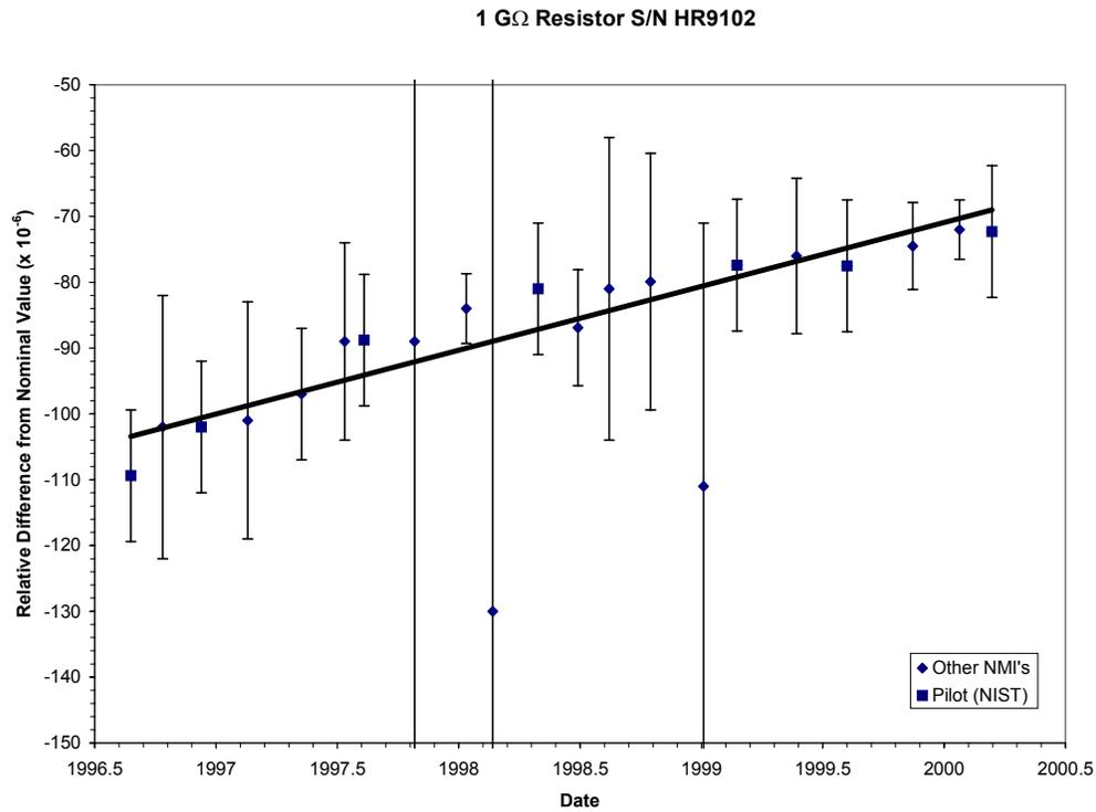
**Figure 6.** Measurements of 1 GΩ standard S/N HR9102 by all participants. Error bars denote individual NMI's expanded relative uncertainty using  $k = 2$ . Least-squares linear regression line based only on the pilot laboratory measurements.
