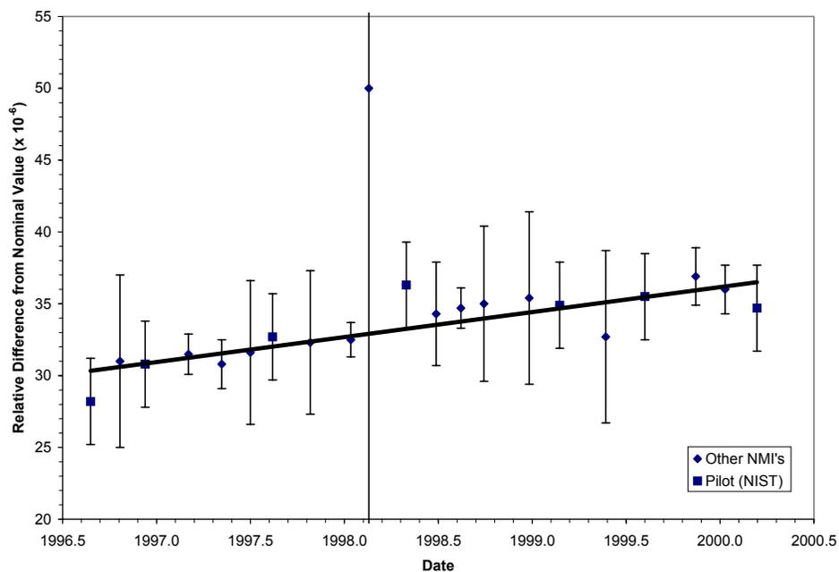
**Figure 1.** Measurements of 10 M $\Omega$  standard S/N HR7550 by all participants. Error bars denote individual NMI's expanded relative uncertainty using  $k = 2$ . Least-squares linear regression line based only on the pilot laboratory measurements.
