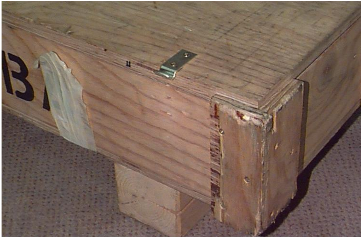
Fig. 3 Damage to shipping box of step gauge
