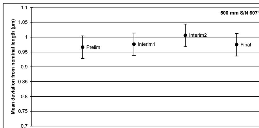
Figure 1(b) Stability of 500 mm gauge block (S/N 6071) during comparison: interim length measurements of the pilot laboratory. Uncertainty bars show standard uncertainty ( $k=1$ ).
