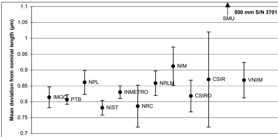
Figure 3(c) Results for the 500 mm gauge block, S/N 3701 (standard uncertainty bars shown).
