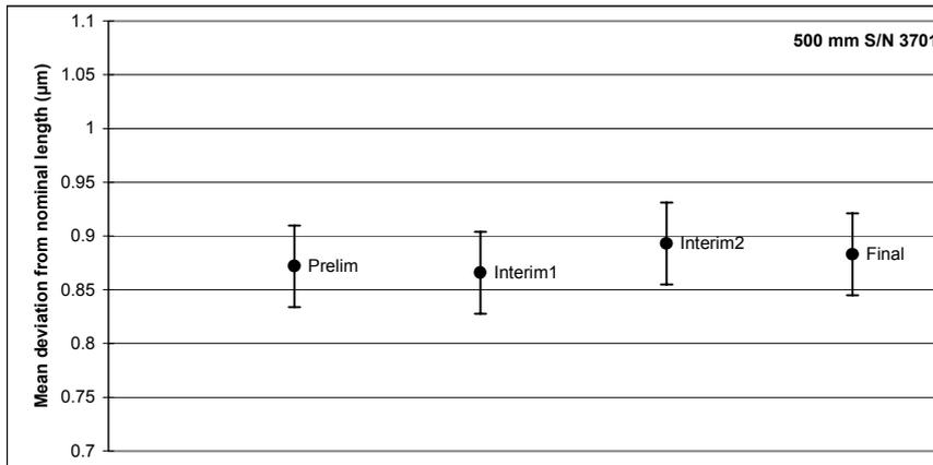
Figure 1(c) Stability of 500 mm gauge block (S/N 3701) during comparison: length measurements of the pilot laboratory. Uncertainty bars show standard uncertainty ( $k=1$ ).
