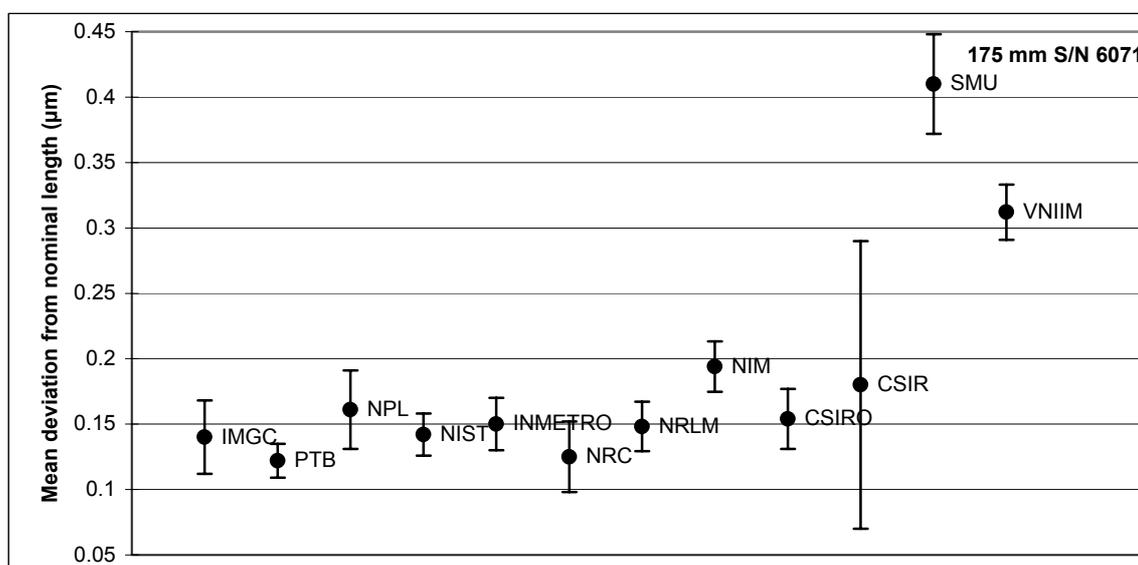
Figure 3(a) Results for the 175 mm gauge block, S/N 6071 (standard uncertainty bars shown).
