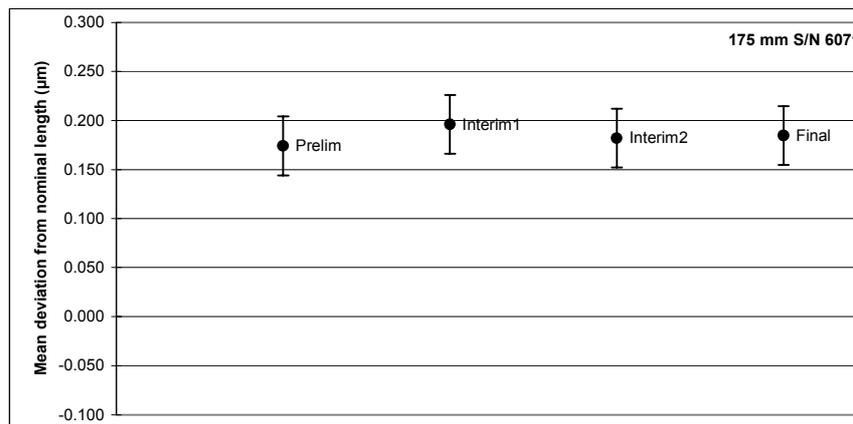
Figure 1(a) Stability of 175 mm gauge block (S/N 6071) during comparison: interim length measurements of the pilot laboratory. Uncertainty bars show standard uncertainty ( $k=1$ ).
