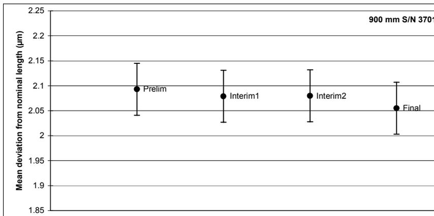
Figure 1(d) Stability of 900 mm gauge block (S/N 3701) during comparison: length measurements of the pilot laboratory. Uncertainty bars show standard uncertainty ( $k=1$ ).
