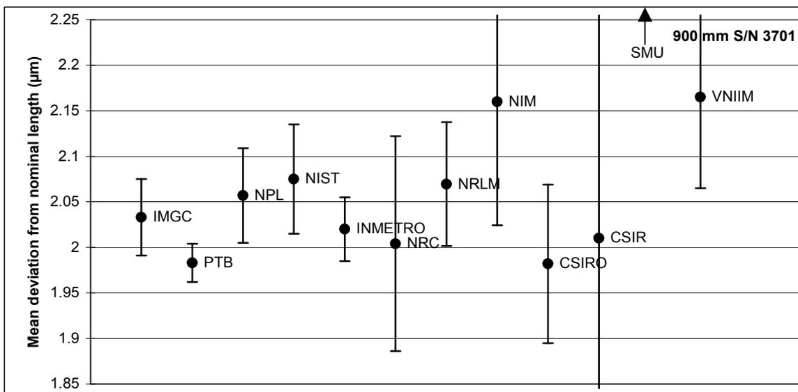
Figure 3(d) Results for the 900 mm gauge block, S/N 3701 (standard uncertainty bars shown).
