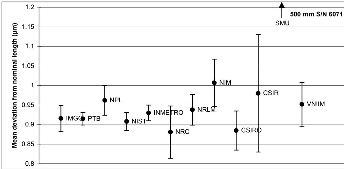
Figure 3(b) Results for the 500 mm gauge block, S/N 6071 (standard uncertainty bars shown).
