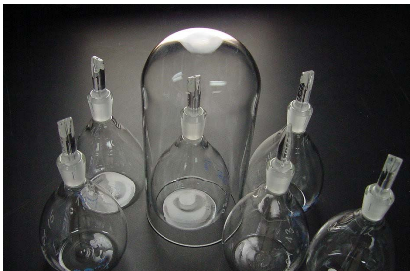
Fig. 2 An image of the Gay-Lussac type pycnometers for volumes of 100 mL
