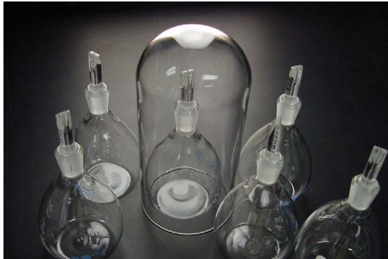
Fig. 7 An image of the Gay-Lussac type pycnometers for volumes of 100 mL
