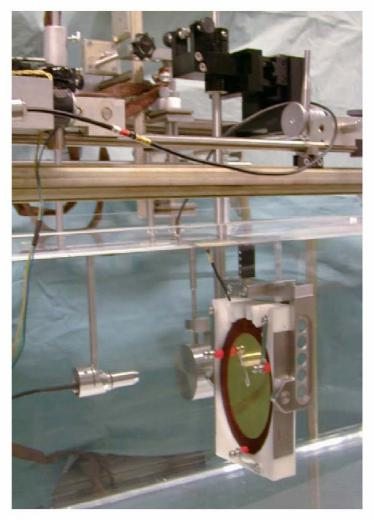
Figure 1. The modified set-up of the reciprocity method used by TNO PG
