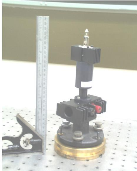
Figure 3.1 Transfer standard lamp with lamp support
