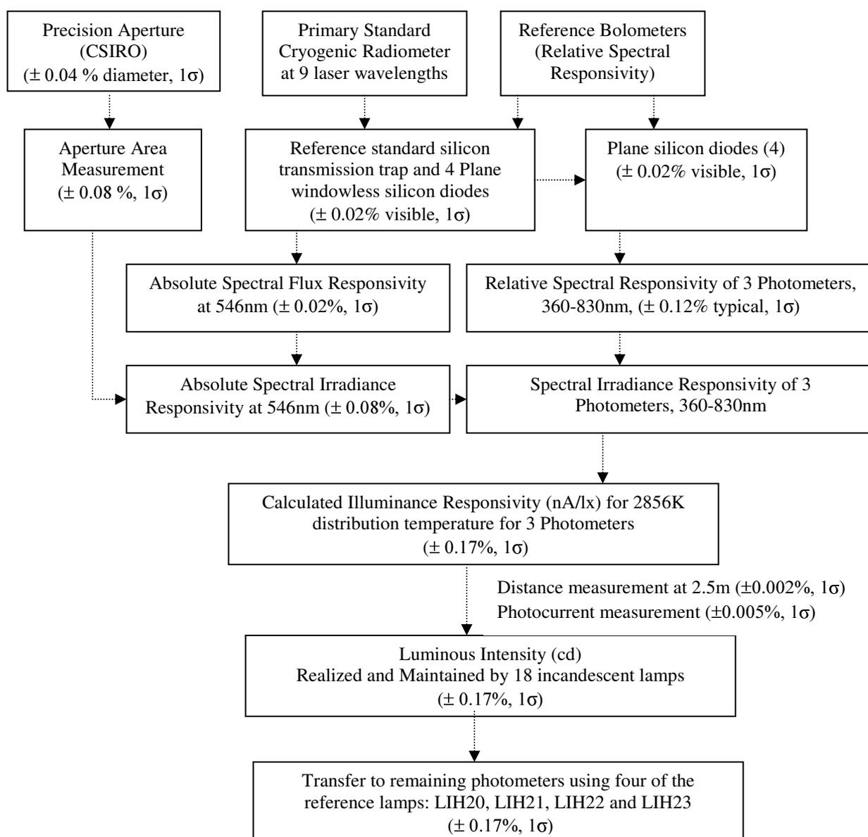
**Figure A.3.2** Traceability chart for realising scales of luminous intensity and luminous response at CSIRO.
