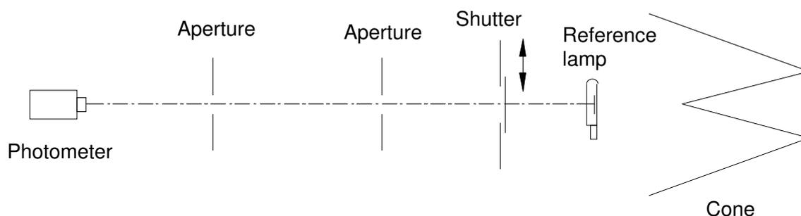
**Figure A.3.1** The set-ups of both measurement for luminous intensity and luminous responsivity is as shown in the figure. The distance between the luminous intensity lamps and the detector calibration plane is fixed at 2.5m.
