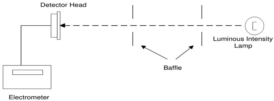
**Figure A.3.4** The set-ups of both measurement for luminous intensity and luminous responsivity at SPRING is as shown in the figure. The distance between the luminous intensity lamps and the detector heads is fixed at 2.5m.
