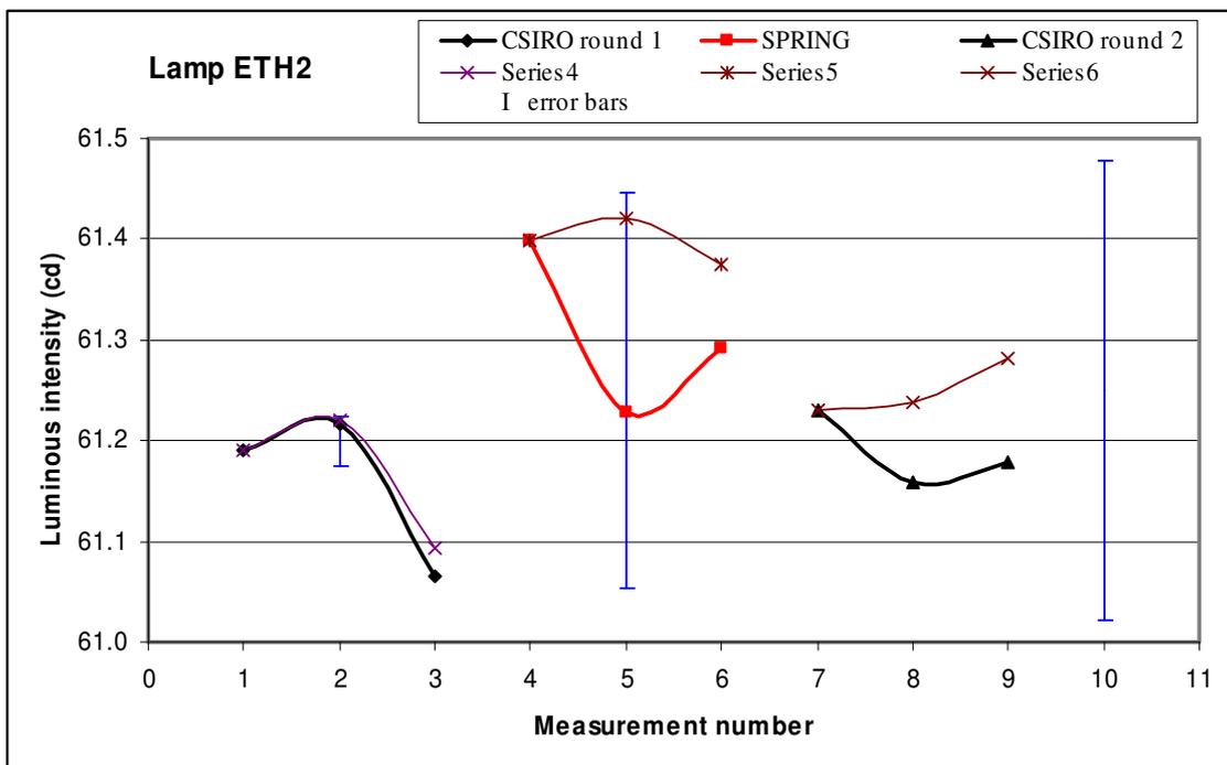
**Figure 5.2** Comparison of measurement results for the lamp ETH2. Finer lines show predicted changes in intensity based on lamp voltage changes. Error bars represent CSIRO random uncertainties, SPRING total uncertainties and combined total uncertainties.
