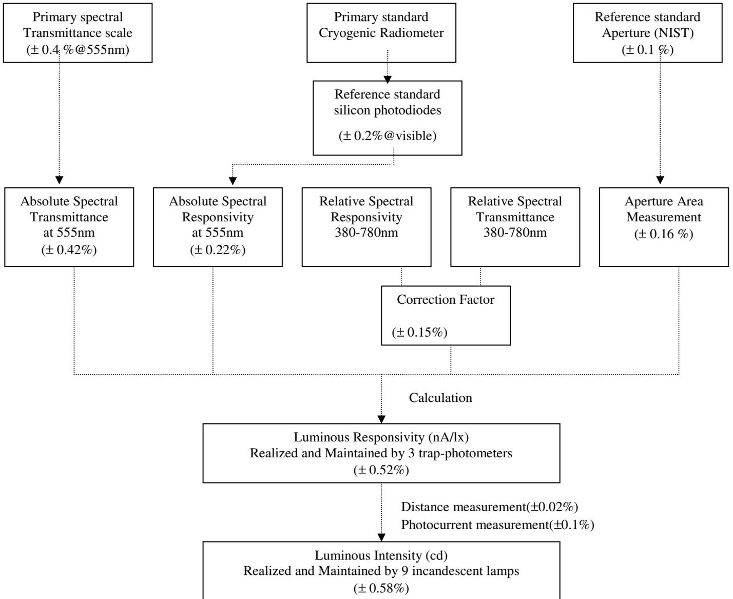
**Figure A.3.3** Traceability chart for realisation of scales of luminous intensity and illuminance response at SPRING.
