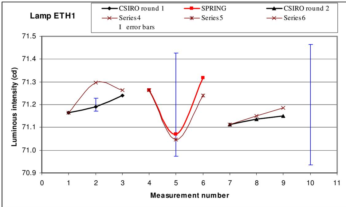
**Figure 5.1** Comparison of measurement results for the lamp ETH1. Finer lines show predicted changes in intensity based on lamp voltage changes. Error bars represent CSIRO random uncertainties, SPRING total uncertainties and combined total uncertainties.
