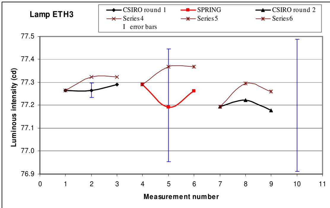
**Figure 5.3** Comparison of measurement results for the lamp ETH3. Finer lines show predicted changes in intensity based on lamp voltage changes. Error bars represent CSIRO random uncertainties, SPRING total uncertainties and combined total uncertainties.
