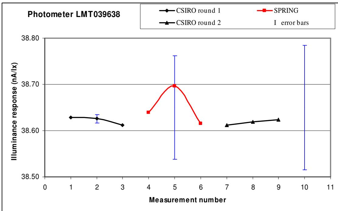
**Figure 5.4** Comparison of measurement results for the photometer LMT039638. Error bars represent CSIRO random uncertainties, SPRING total uncertainties and combined total uncertainties.
