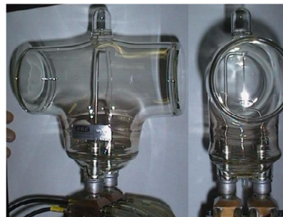
Figure 1 The GEC high-stability vacuum tungsten-strip lamp (side and front view).
