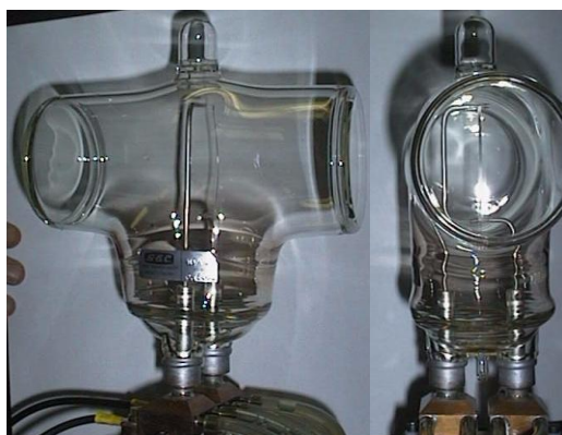
Figure 2 The GEC high-stability vacuum tungsten-strip lamp in side and front view.
