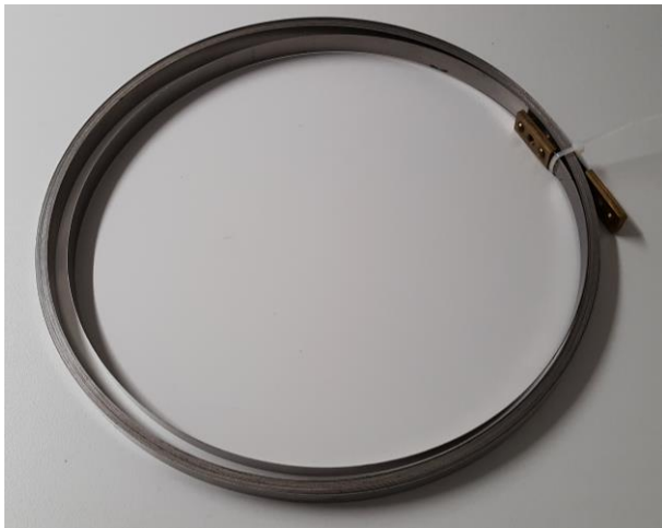
Figure 2 – 10 m tape with 5 millimeter graduation (4909 PTB 01)
