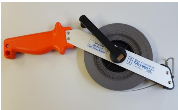
Figure 4 – 50 m tape with millimeter graduation (5.42-0917)
