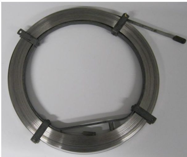
Figure 3 – 50 m tape with meter graduation (5060 PTB 06 No.3)
