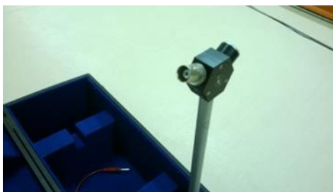
Connectors of the chamber LS-01: BNC (female) and Lemo.
