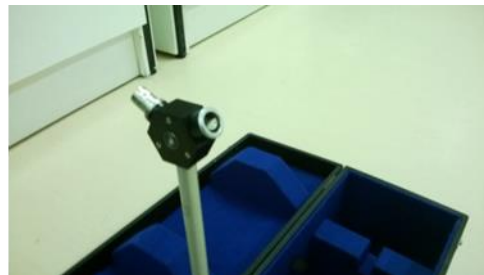
Connectors of the chamber LS-01: BNC (female) and Lemo.
