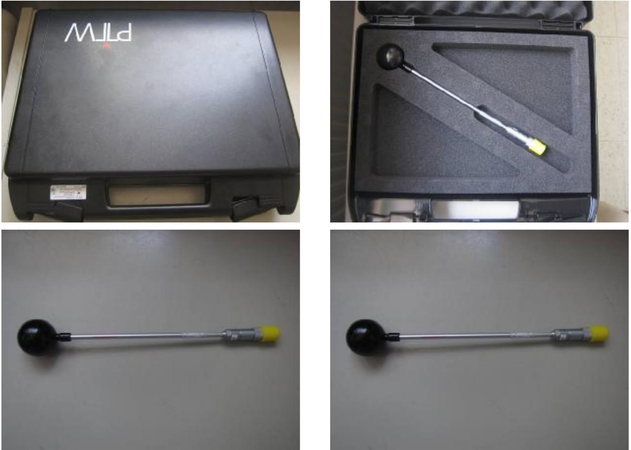
**Figure 5** Ionization chamber PTW 32005 TK-30, SN 000136 and case
