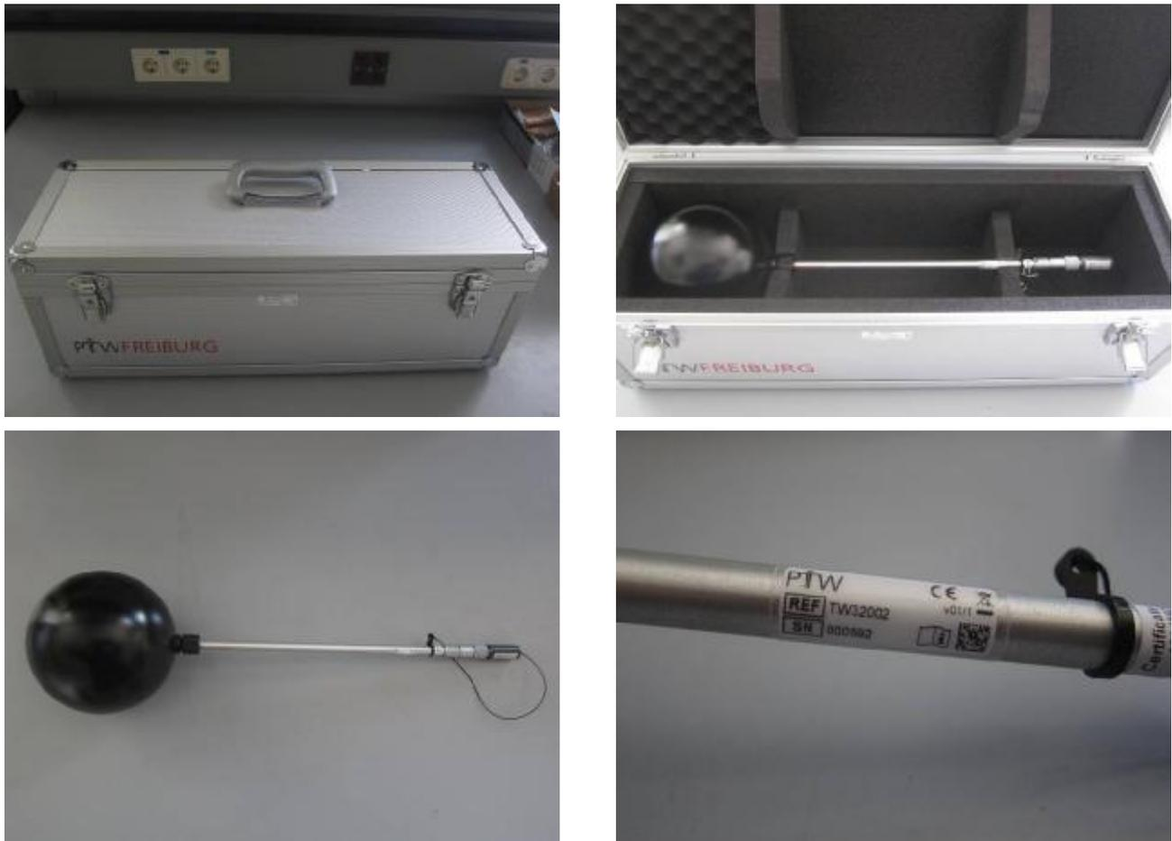
**Figure 6** Ionization chamber PTW 32002 1 I, SN 000592 and case
