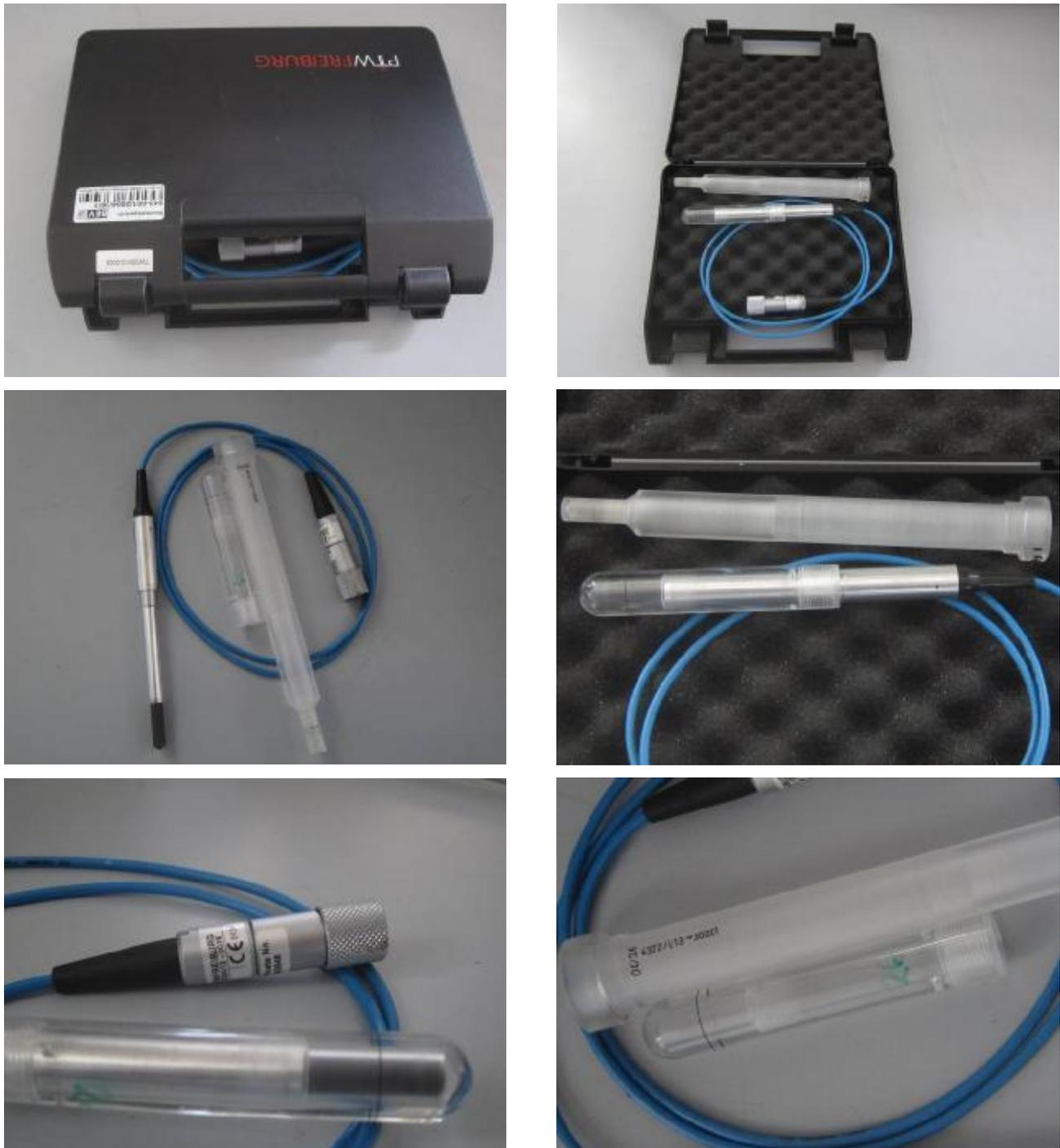
**Figure 3** Ionization chamber PTW T30012, SN 0026, including PMMA-Sleeve 4322/U13 and case
