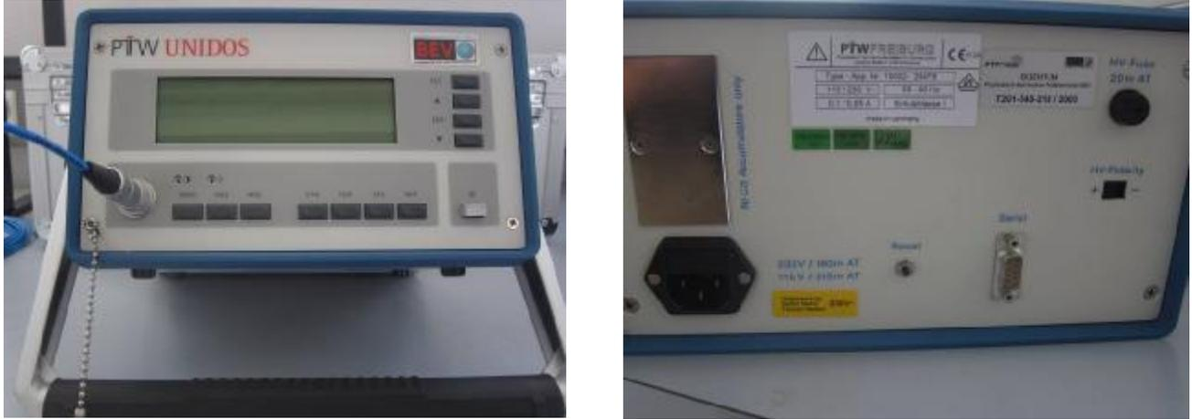
**Figure 1** Electrometer PTW UNIDOS 10002, SN 20478
