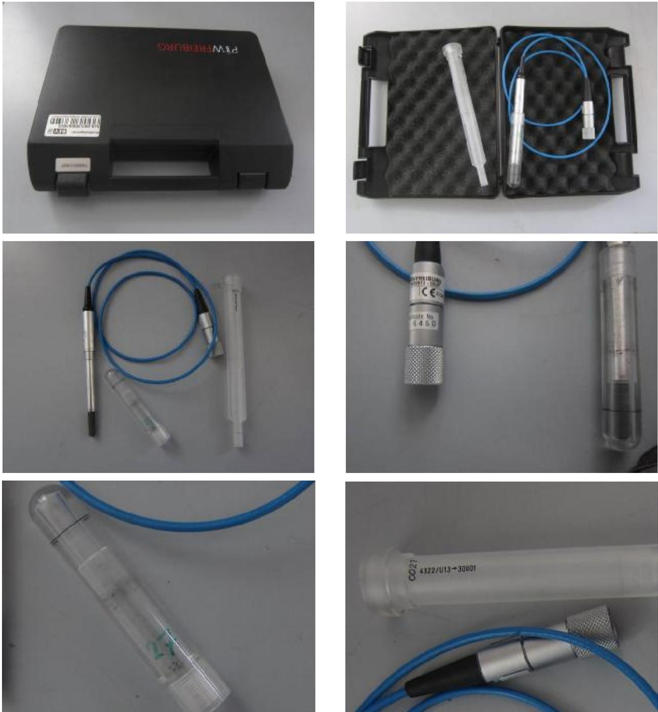
**Figure 4** Ionization chamber PTW T30012, SN 0027, including PMMA-Sleeve 4322/U13 and case
