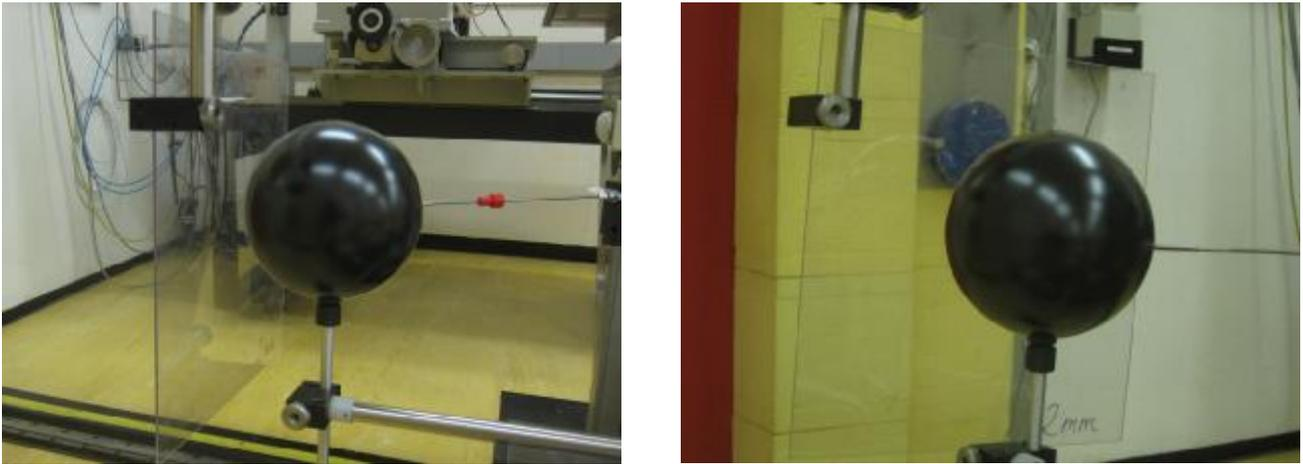
**Figure 16** Air kerma, radiation protection level Cs-137, ionization chamber PTW 32002 1 I, including 2 mm PMMA plate and temperature sensor
