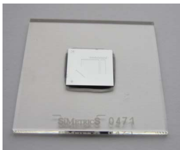
Fig. 5 The SiMetrics depth setting standards consist of a glass plate with the bonded silicon chip on it and an engraved serial number
