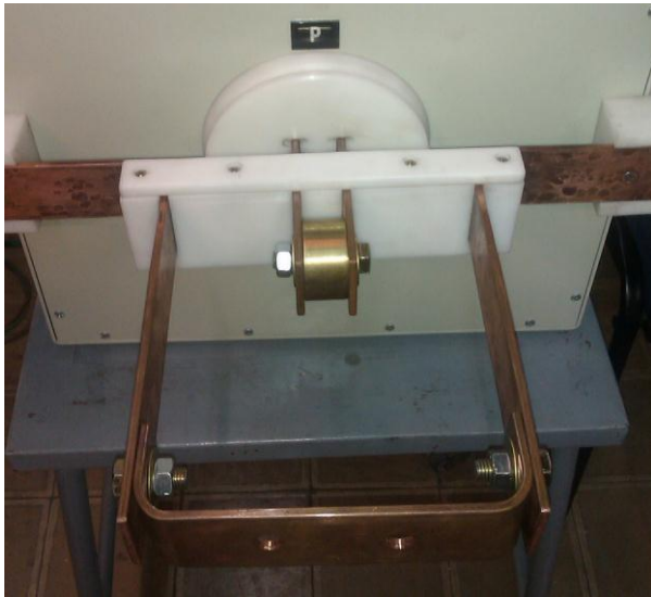
Fig. 6. Auxiliary bars for parallel connexion.
