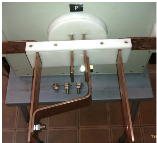
Fig. 7. Auxiliary bars for series connexion.
