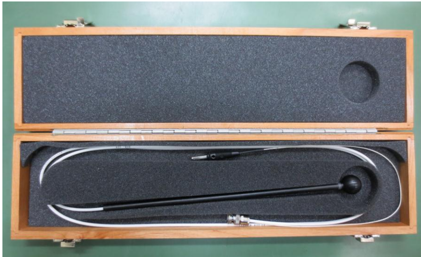
Fig. 1. A spherical Exradin A3 chamber. No build-up cap is provided since the wall is 2.5 mm-thick. The length of the stem is 28.5 cm and the outer diameter of the chamber is 23.5 mm. Bias is supplied with banana plug and signal is measured with BNC.
