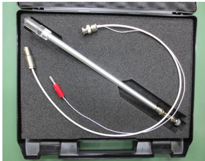
Fig. 2. A cylindrical PTW 23331 chamber. A 3 mm-thick PMMA build-up cap is put on the chamber. The length of the stem is 32.7 cm and the outer diameter of the chamber with a build-up cap is 15.0 mm. Cable can be linked either with a tri-axial connector or using an adapter for connecting the tri-axial connector to BNC-banana plug.
