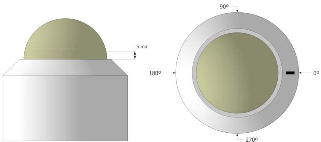
Figure 3 – Measurement plane and alignment of the glass hemisphere.
