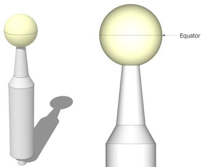
Figure 4 – Measurement plane of the sphere.
