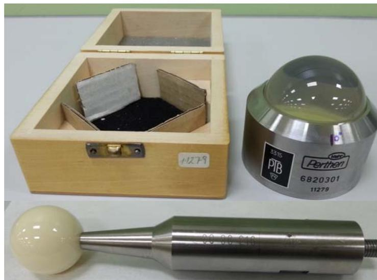
Figure 2 – Glass hemisphere (Perthen 11279) and sphere (Saphirwerk 30-96-216)
