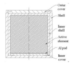
Source core (active element) size: Φ19×18mm Source core preparation: ceramic technology preparation. Mixing AmO<sub>2</sub> with BeO, and after 6 hours of 1600°C~1700°C high temperature burning, the ceramic source core with high density, high hardness, high stability of is made. Source cre weight: 7.4g
