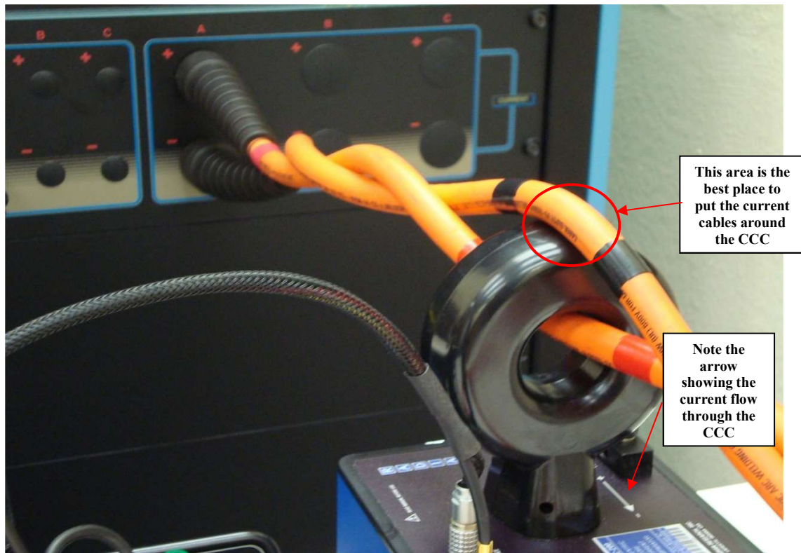
Figure 5. Current cables around the Concentric Current Comparator of the RD-22-432.
