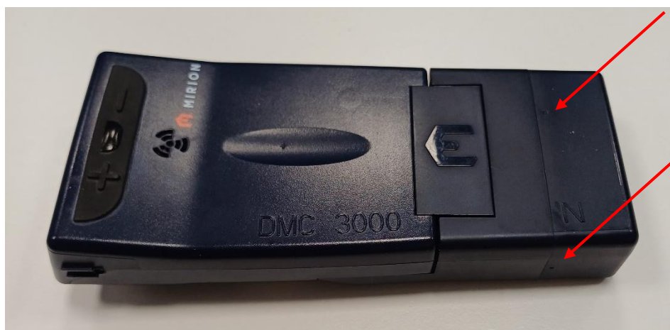
Figure A2. DCM3000 instrument. Reference points are marked with red arrows.
