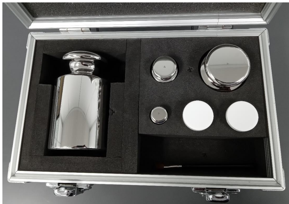
Fig. 1: BSJ travelling standards.
