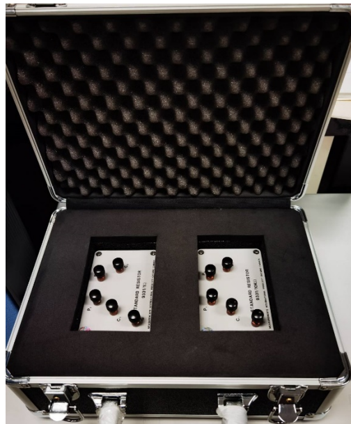
Figure 3. Packed standard resistors in their protective luggage
