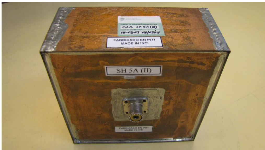
Figure 1 Physical layout of the 5 A shunt.
