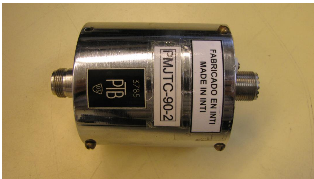
Figure 2 Physical layout of the thermal converter PMJTC-90-2.
