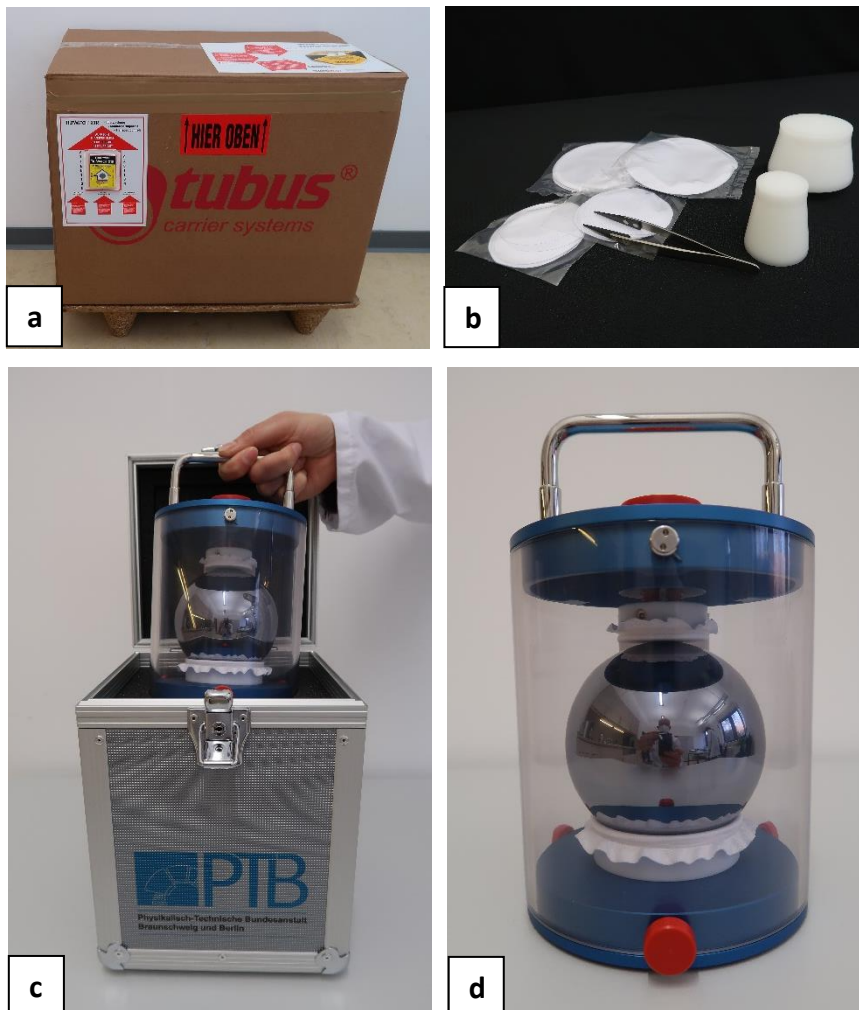
Figure 1 a - d. For transportation, the silicon sphere will be shipped in a cardboard box on a pallet (a), additionally enclosed are auxiliary tools (b). For this purpose, the silicon sphere is placed in an aluminum carrying case (c) and in a transport container (d).
