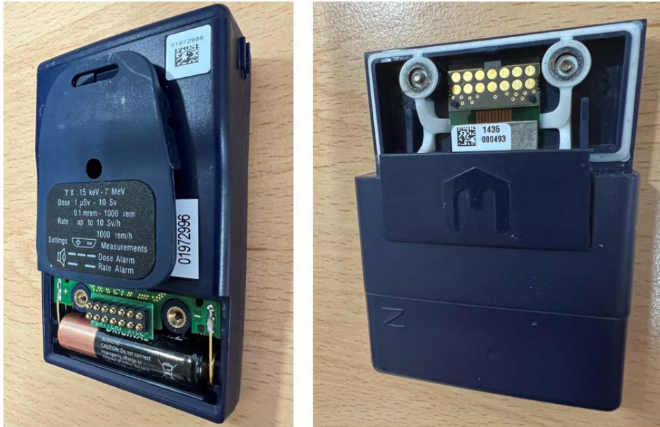
Fig. 3. DMC3000 S/N 09172996 (left) and neutron module S/N 000493 (right)
