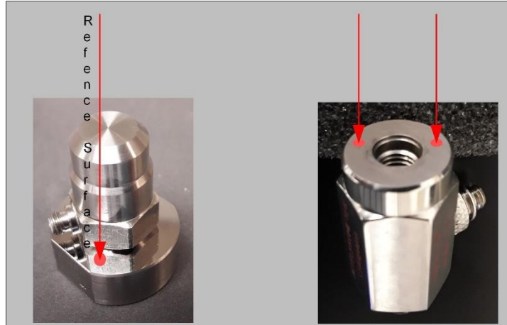
Figure 1: Reference surfaces indicated for the Brüel & Kjær 8305-001 accelerometer complete with adaptor and the ENDEVCO 2270
