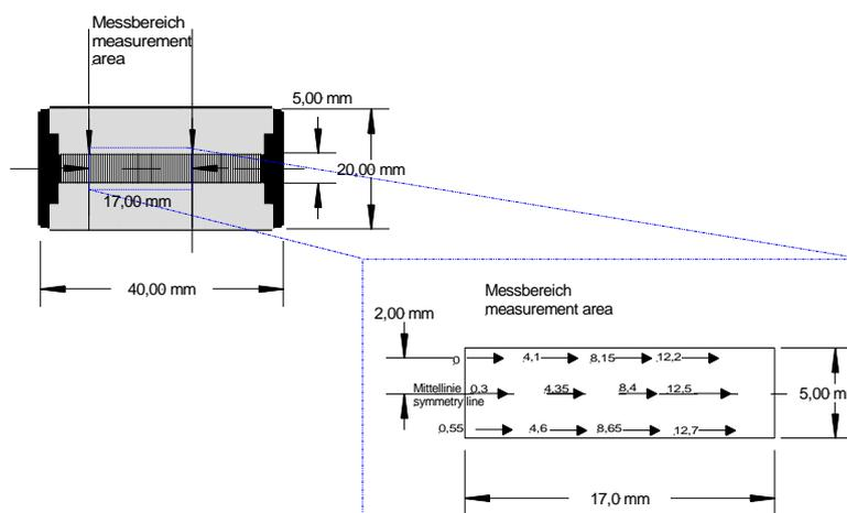
Figure 6 - The area of measurement shows the starting points and traversing direction of the respective traversing lengths of **5.6 mm**.
