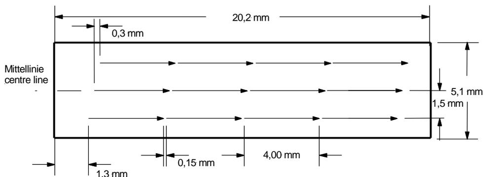
Figure 4 - The area of measurement shows the starting points of the respective evaluation lengths of **4.0 mm**.
