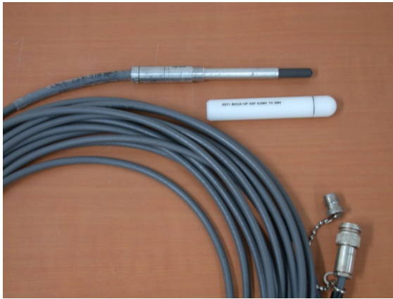
NE 2571 chamber (S/N 3025, non-waterproof)
