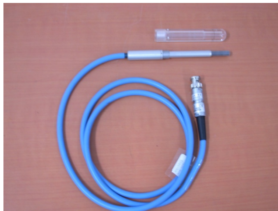
PTW 30013 chamber (S/N 0348, waterproof)
