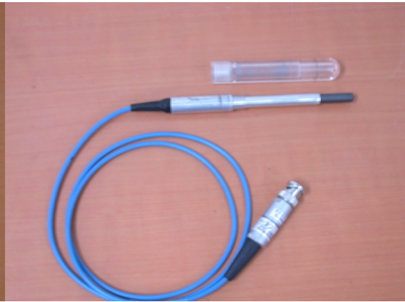
PTW 30001 chamber (S/N 2340 non-waterproof)
