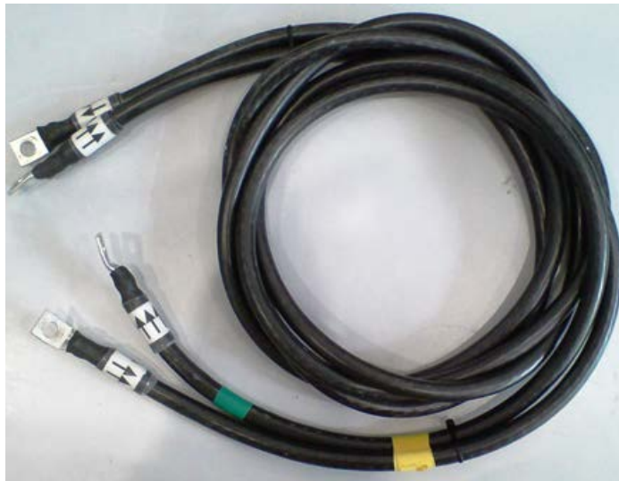
Figure 4 Current cables for connection travelling standard RD-33-332
