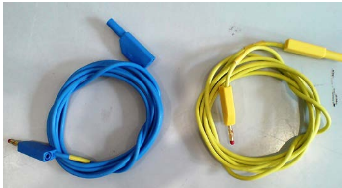
Figure 5 Voltage cables for connection travelling standard RD-33-332
