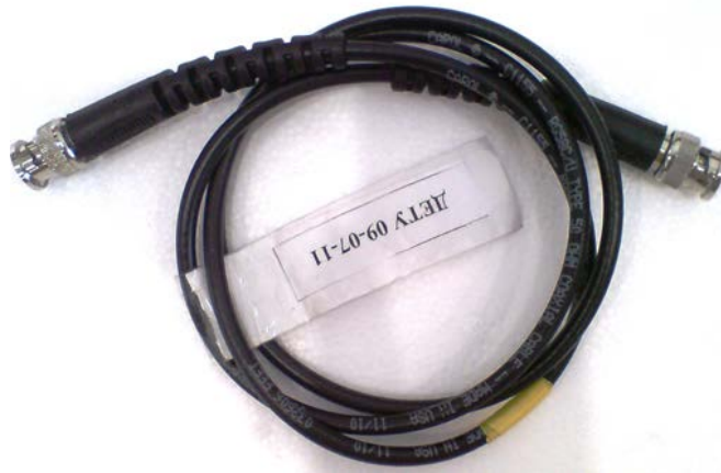
Figure 6 Pulse cable for connection travelling standard RD-33-332
