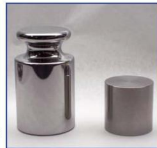
Figure 3: 1 kg of Stainless Steel compared with 1 kg of platinum-iridium
