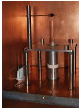
Figure 3. HPGe detector with the ampoule and the ^{241}\text{Am} source.
