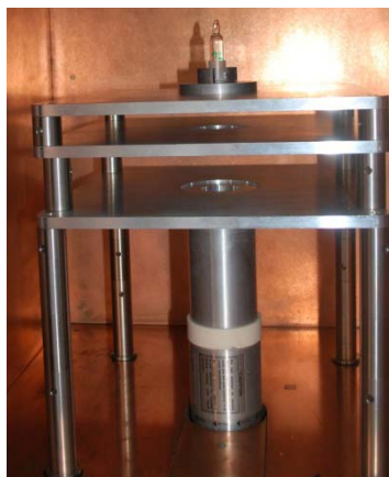
Figure 5. Radon ampoule measurement setup with a HPGe detector.
