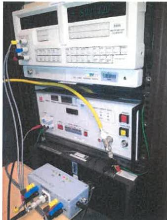
Figure 4. Calibrator & Switch Box
