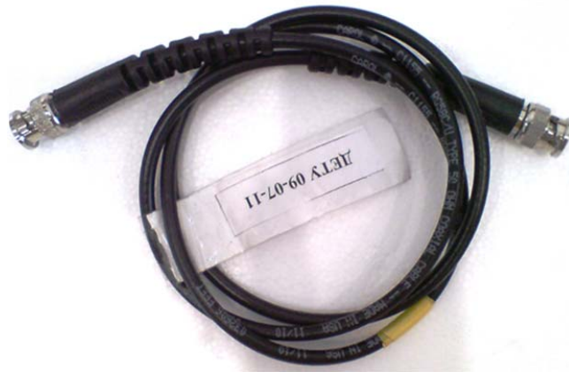
Figure 6 Pulse cable for connection travelling standard RD-33-332
