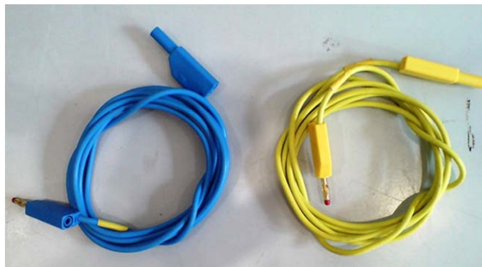
Figure 5 Voltage cables for connection travelling standard RD-33-332
