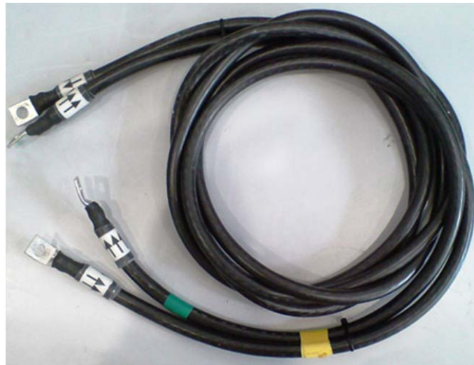
Figure 4 Current cables for connection travelling standard RD-33-332
