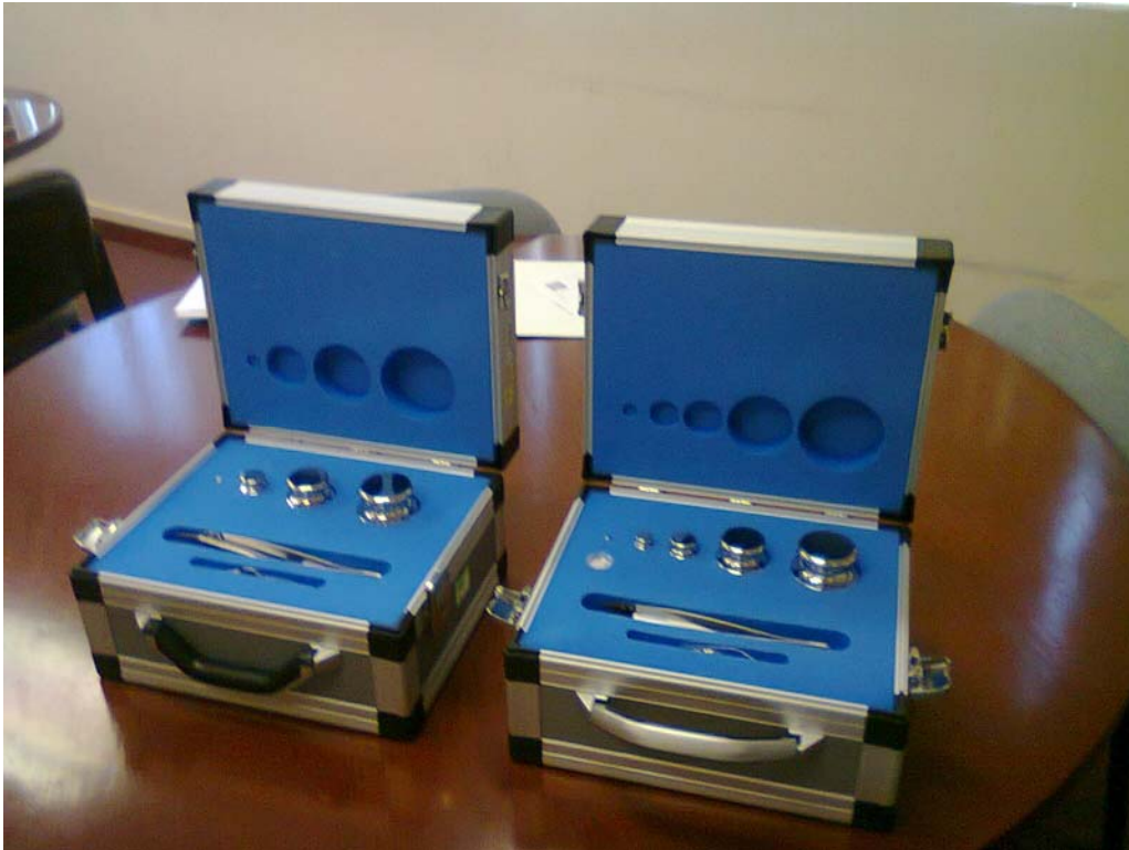
Fig. 2. Sets for the Mass and Volume comparisons, both sets in individual aluminum cases.
