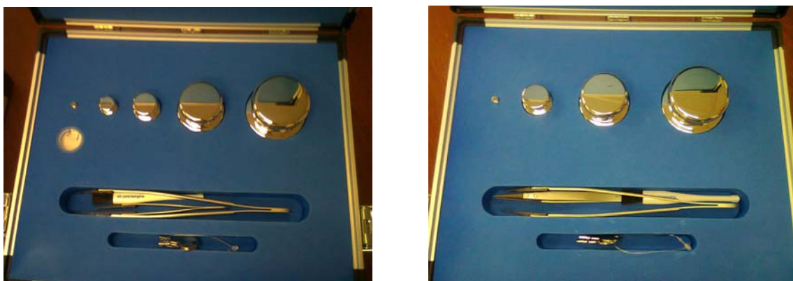
Fig. 1. SET 1 (left) for the mass comparison and SET 2 (right) for the volume (and density) comparison.
