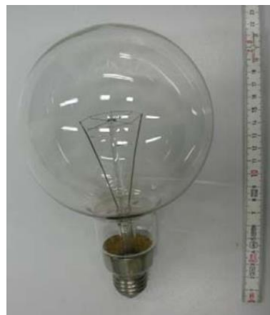
Figure 1: Standard luminous flux lamps of UME (Polaron LF200W) used within this comparison.
