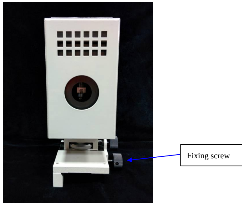
Figure 2. Deuterium Lamp in housing. Front view.
