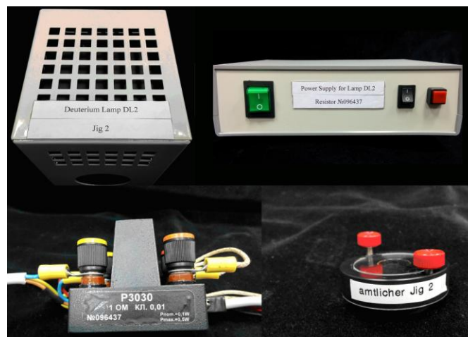
Figure 1. The identification number and labels on lamp (up left), power supply (up right), shunt resistor (down left) and alignment jig (down right)
