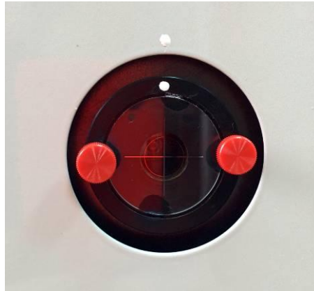
Figure 4. The Jig has to be connected to the internal (black) screen of the lamp housing in that way that the mark on the jig coincides the mark on the housing
