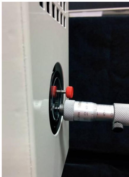
Figure 5. The front surface of the jig glass window is used as the reference plane for the distance measurement
