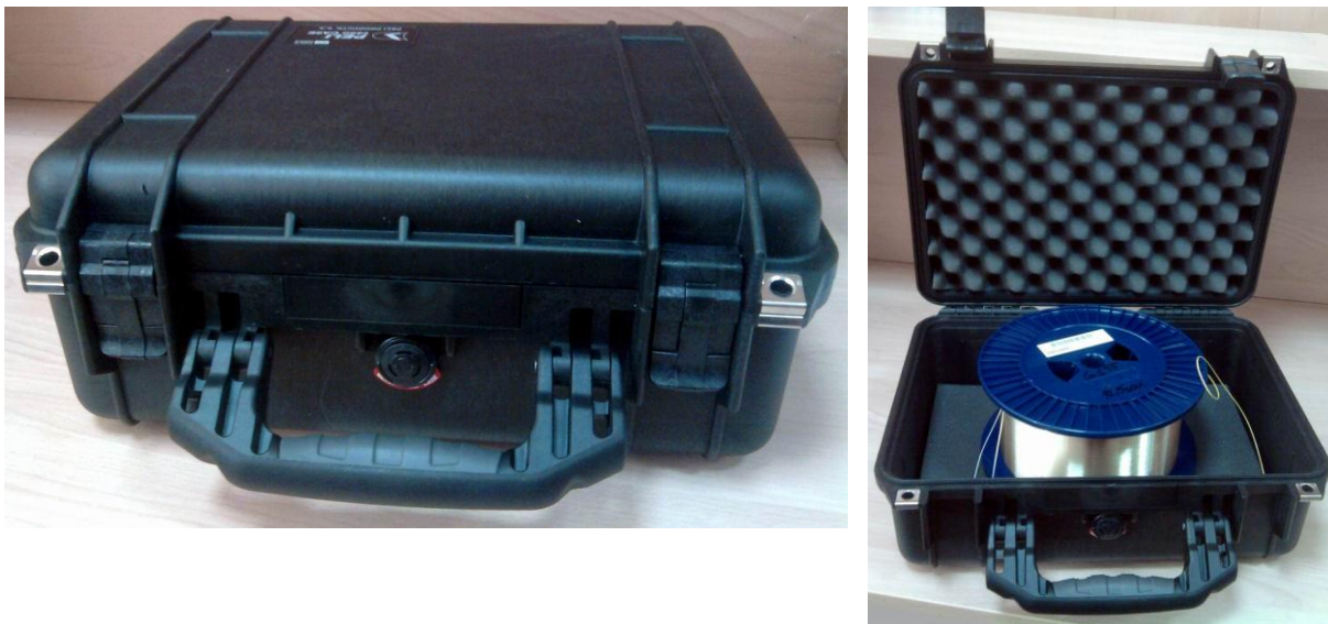
Fig. 1. Reference Fibres mounted in a thermal enclosure.
