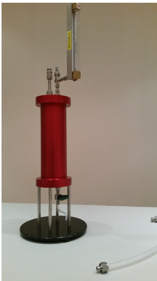
Fig.8: Condensation trap assembled with flowmeter
