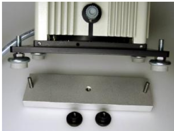
Figure 5. Holder for the lamp systems. The lamps can easily be replaced and fixed on that adapter.
