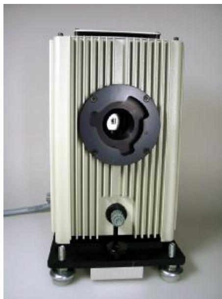
Figure 2. The lamp housing includes a connector for electrical measurements at the back (not shown), a base plate to be placed on a flat surface and a specially designed opening that allows the lamp jig and the monitor detector to be connected reproducibly to the housing.
