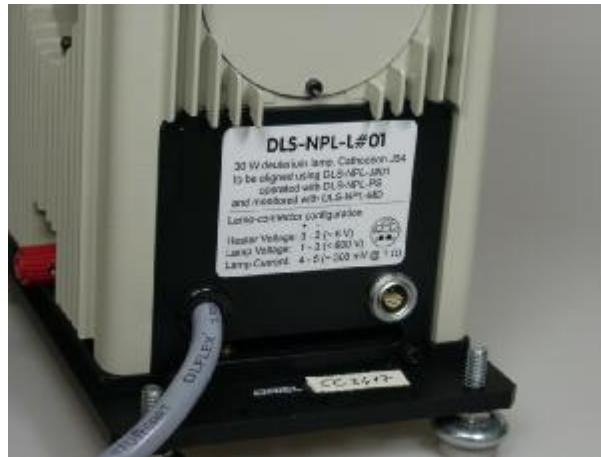
Figure 6 Connector at the lamps back to measure the electrical parameters of the lamp: Pin 1-2, ...
