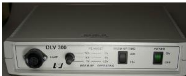
Figure 1 Power supply DLV300 – The settings for preheating time (20 s) and heating level (10V/6V) have to be as shown on the picture. These settings and the notation of the power supply are printed on a label on top of the power supply.
