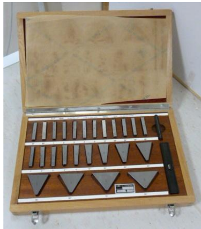
Figure 1 : Image of the angle block box. There 25 angle blocks, only the 10", 5', 30', 5°, 30° angle blocks will be measured. The others should be kept untouched under grease protection.
