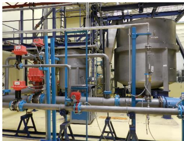
Fig. 3: Front view of the static weighing system at CENAM Primary System for Water Flow
