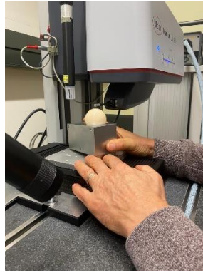
Figure 2. Measuring Instrument Calibration using Sphere Artefact
