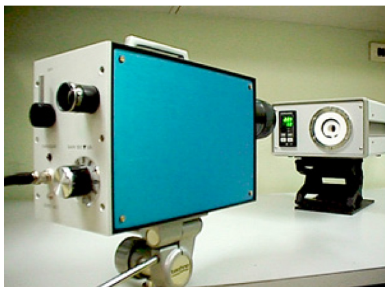
Figure 1: The Transfer Standard thermometer INRiM – TS1.
