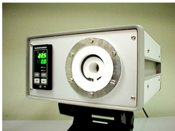
Figure 2: INRiM zinc fixed-point blackbody source.
