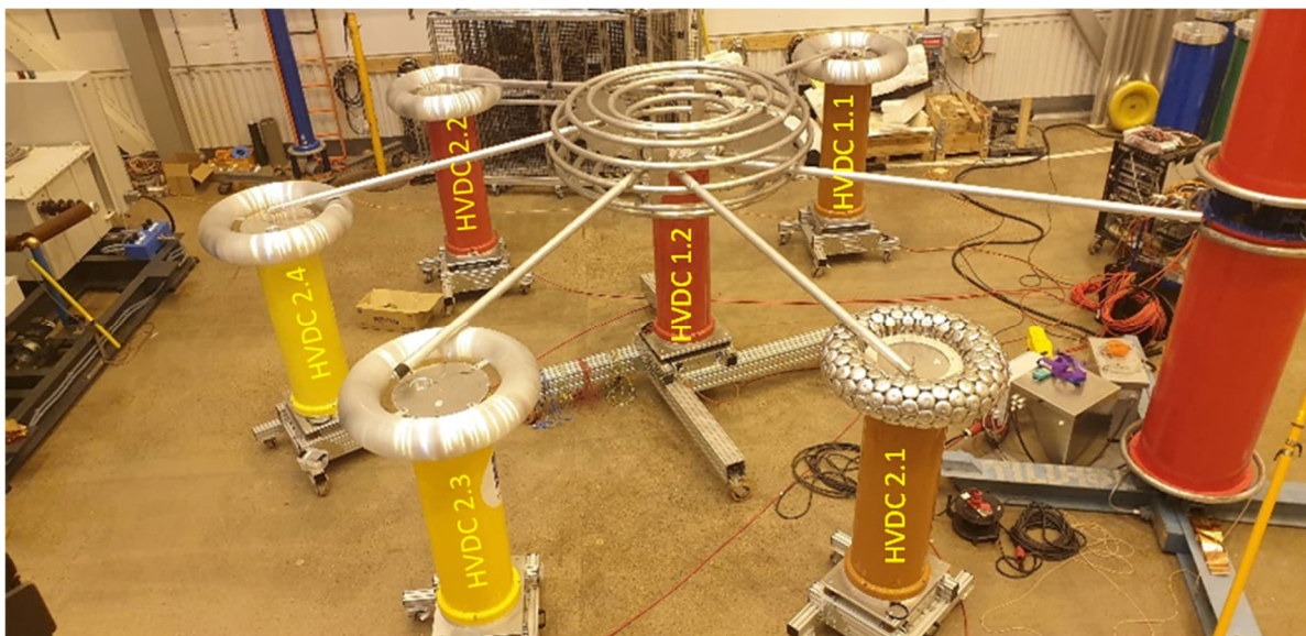
Figure 1 The five high voltage dividers around a sixth one used as transfer divider during EURAMET.EM-S46 DC ratio comparison. The setup was used in that DC ratio comparison, and it is not representative for this resistance comparison.
