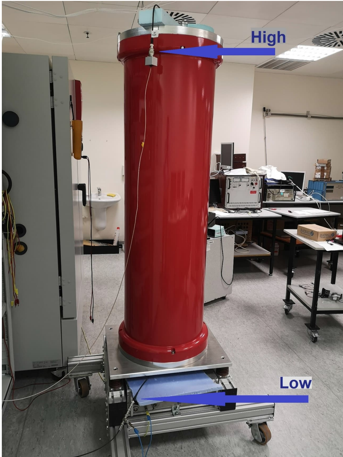
Figure A.2.2 2 G \Omega resistor connection of HVDC divider (the model of HVDC 2.2-LV2)
