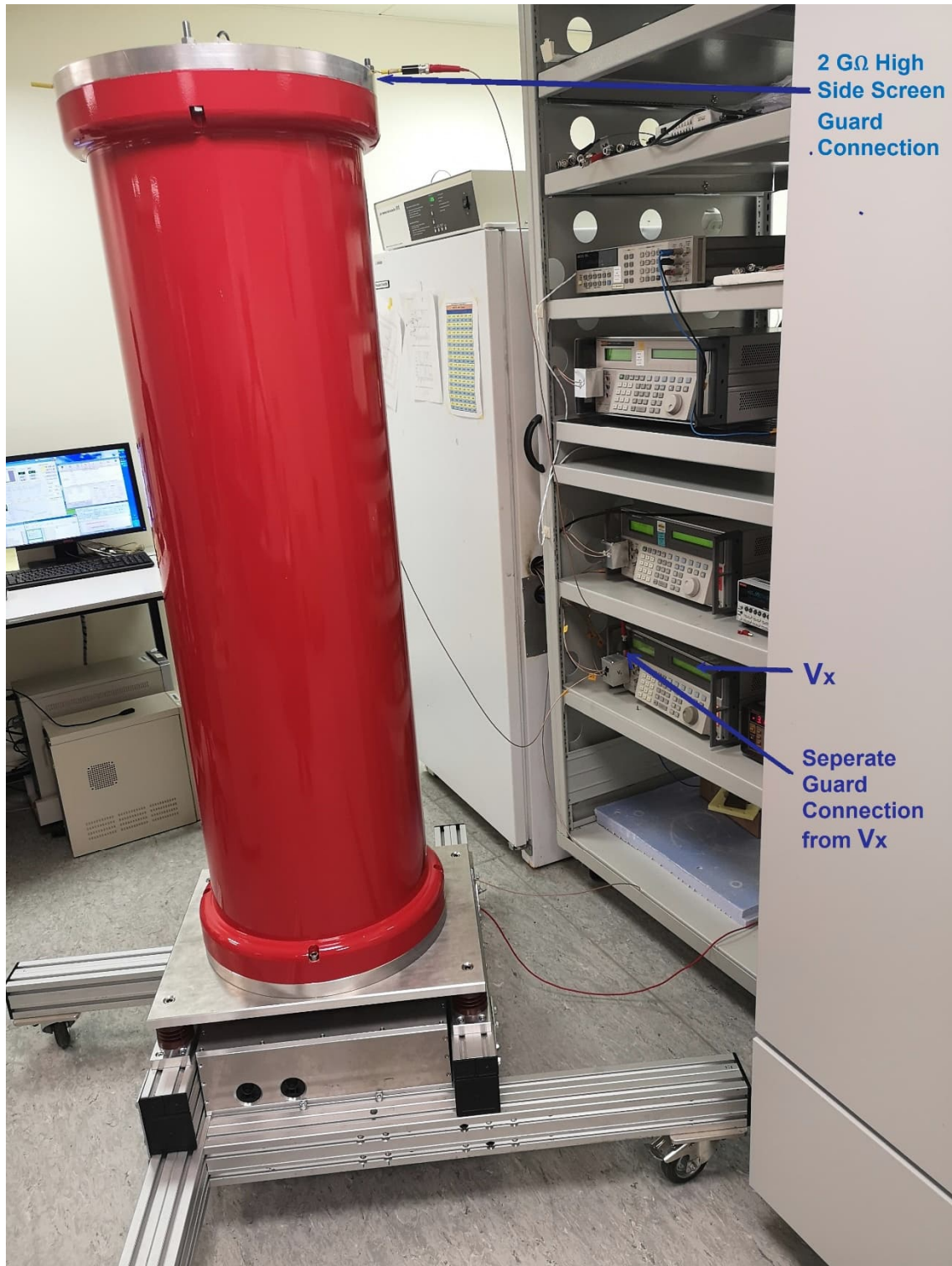
Figure C.3. High Voltage Divider HVDC2.2 2 GΩ Resistor High Voltage Side Connections
