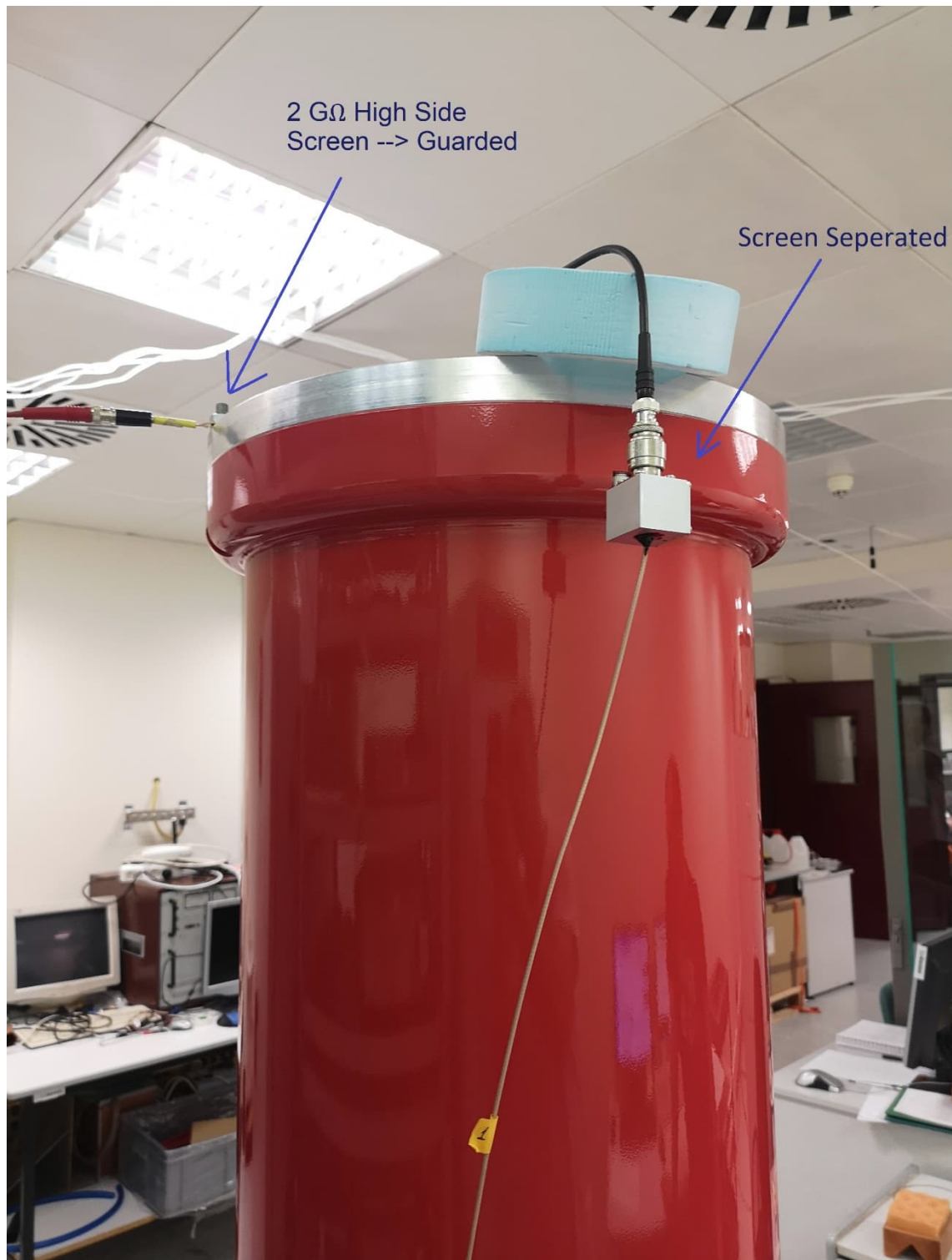
Figure C.2. High Voltage Divider HVDC2.2 2 GΩ Resistor High Voltage Side Connections
