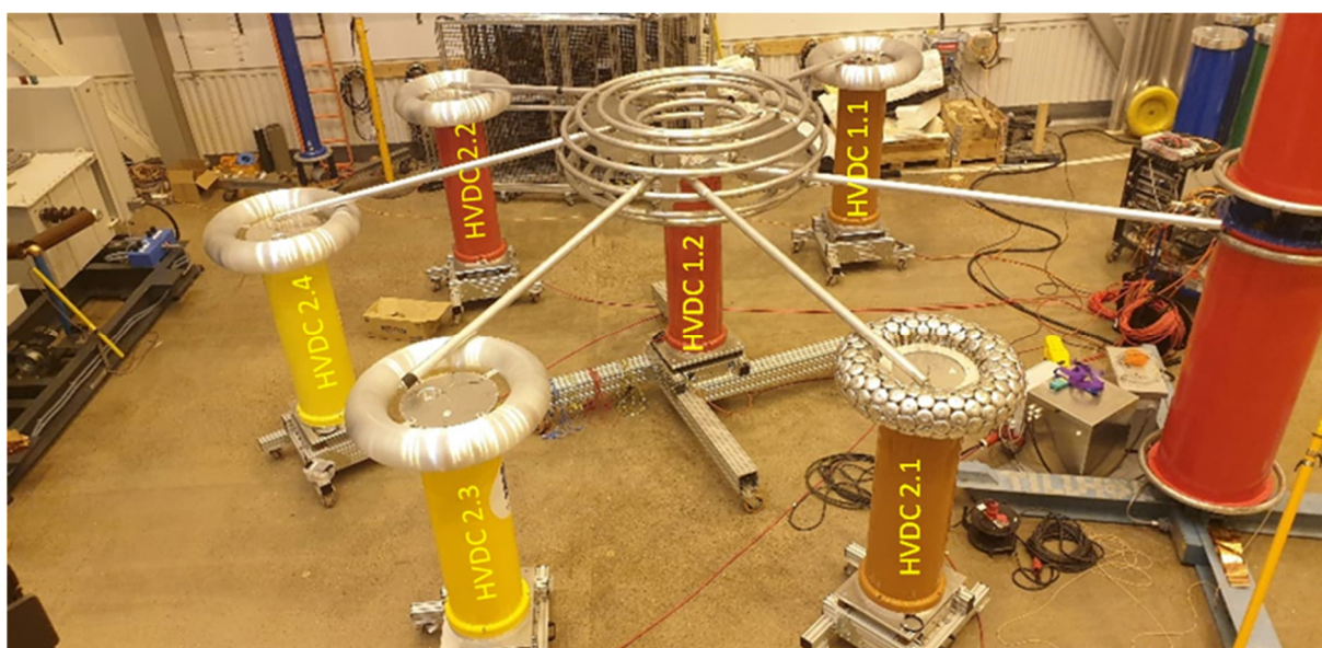
Figure 1 The five high voltage dividers to be compared (HVDC1.1, HVDC2.1, HVDC2.2, HVDC2.3, and HVDC2.4) were set around a sixth transfer divider used as central divider (HVDC1.2) in substitution method.
