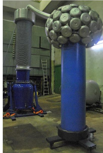
Picture 8 - SE “Ukrmetrteststandard” primary standard for electric capacitance  $C$  and
