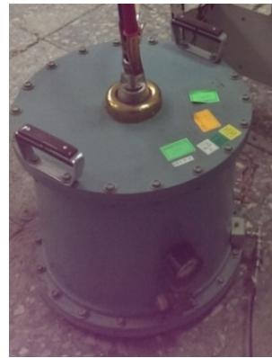
Picture 7 - GEOSTM capacitor VGK-2
