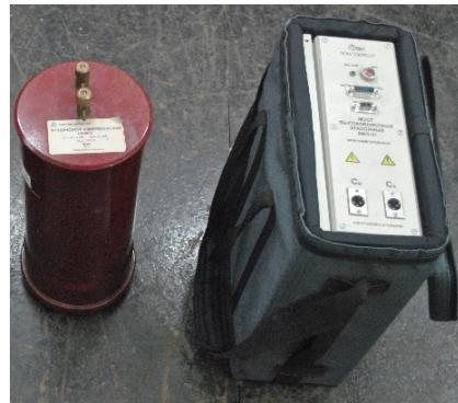
a) Vacuum capacitor SA 60002 and standard high voltage      b) Gas-filled capacitor MSR-600
