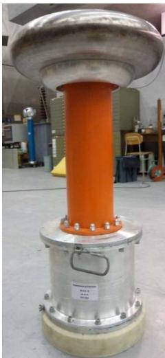
a) High voltage standard capacitor KVE-150;
