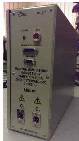
b) Module for measuring the capacitance and loss dissipation factor ( $\tan \delta$ ) MV-capacitor – MVE bridge
